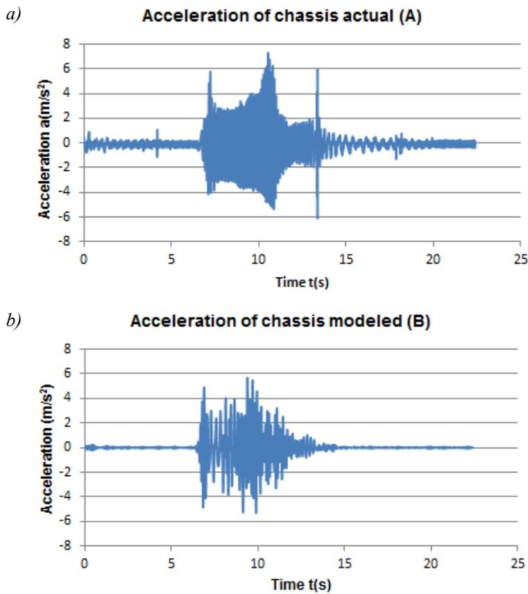
Fig. 7. Comparison of the values of vertical body acceleration: a) actual results, b) modelled results
