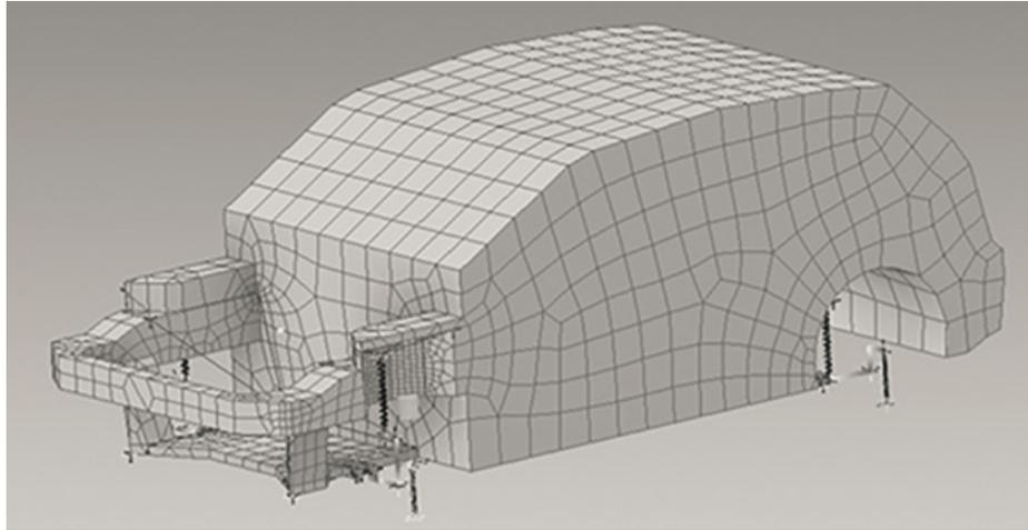
*Fig. 2. Discret model of the car body*
