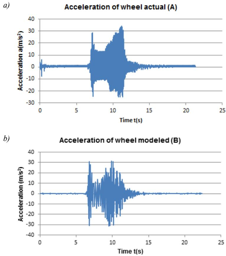
Fig. 6. Comparison of vertical wheel acceleration: a) actual, b) modelled
