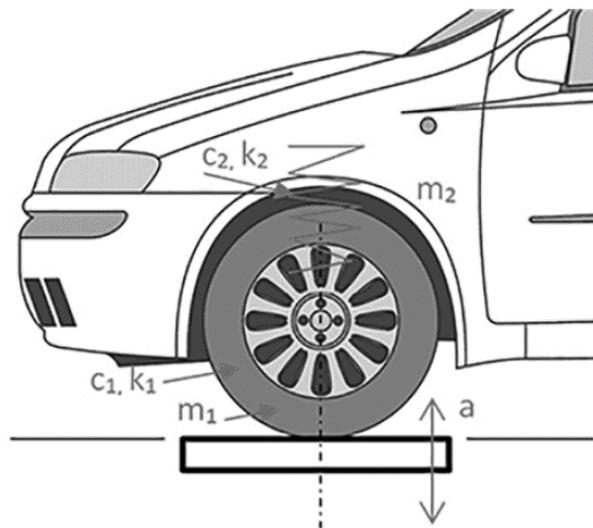
Fig. 1. Diagram of vibrating system
