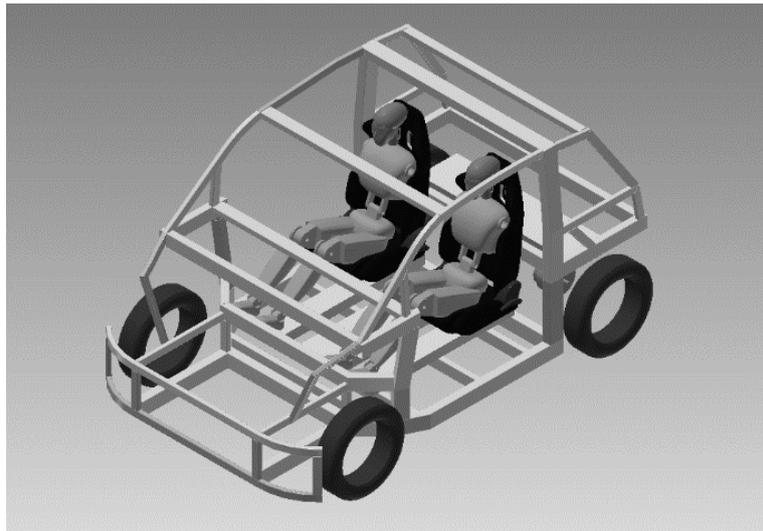
Fig. 9. Prototype of the structural elements of the electric vehicle
