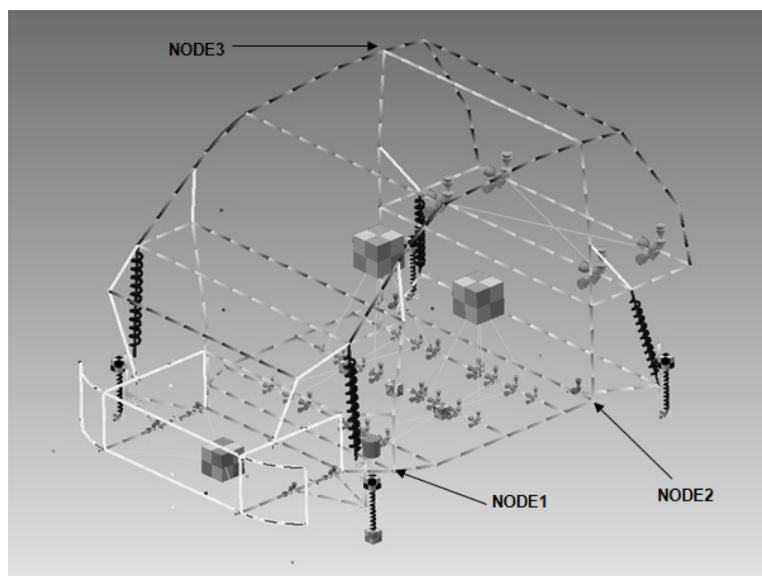
Fig. 10. Vehicle framework presented as a numerical model
