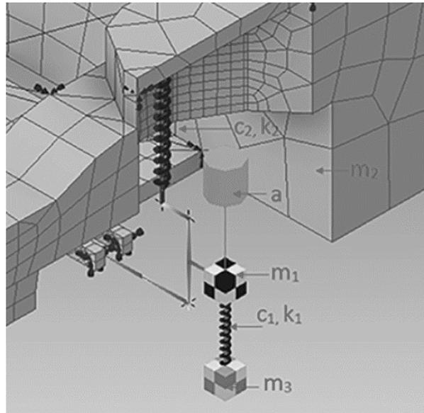
Fig. 4. Diagram of the model of front suspension
