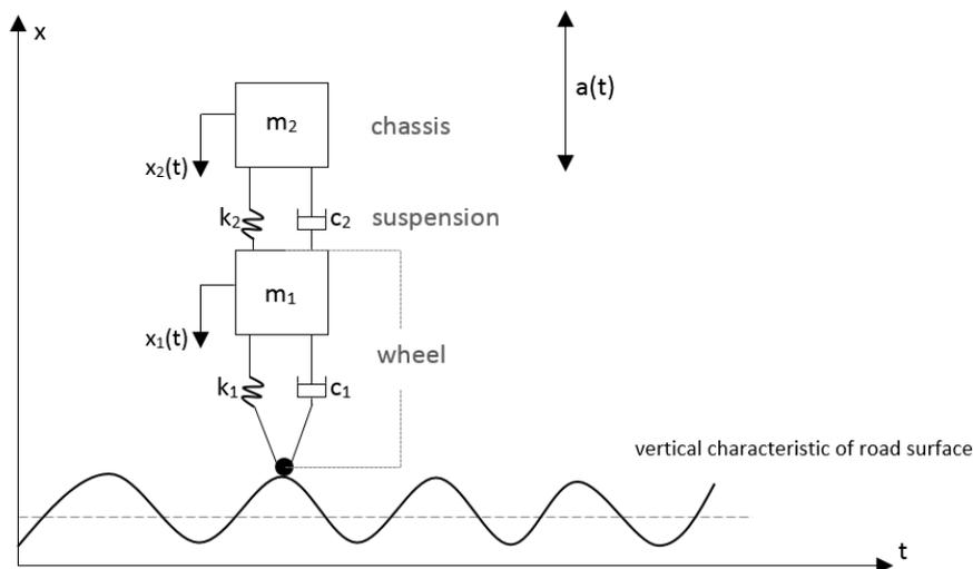
*Fig. 3. Vibrating model with two masses accompanying acting kinematic forces*
