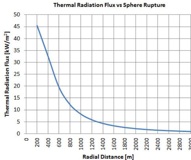
Fig. 5. Thermal Radiation versus Horizontal Distance ( $L$ ) for Sphere Fireball
