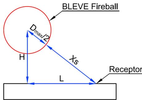
Fig. 4. Geometry for BLEVE Thermal Flux [19]
