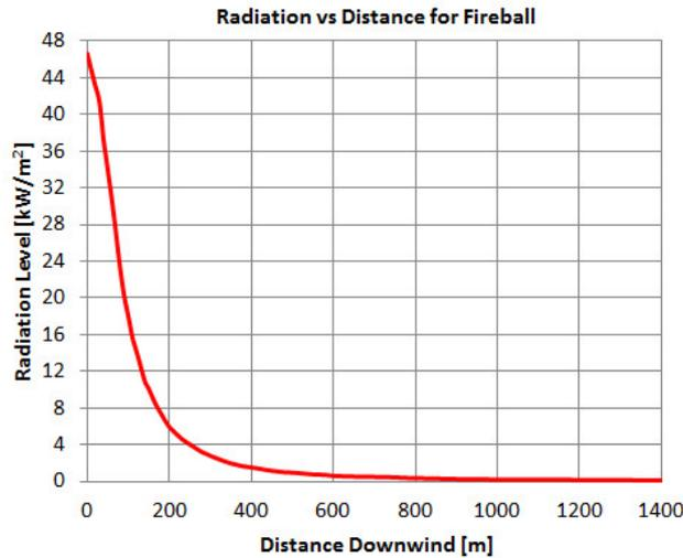
Fig. 6. Thermal Radiation versus Horizontal Distance (L) for Bullet Fireball
