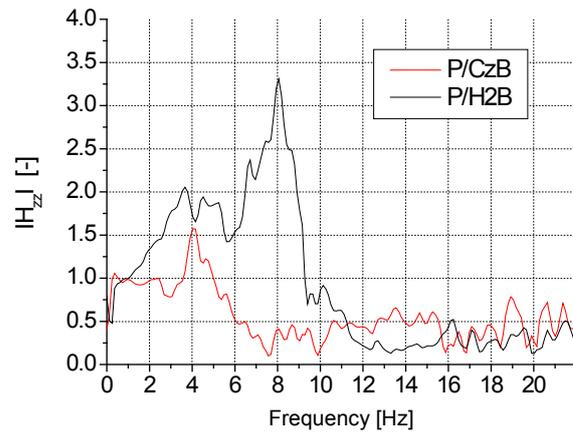
Fig. 12. Absolute acceleration transmittance values (floor-thorax): a comparison between P/CzB and P/H2B
