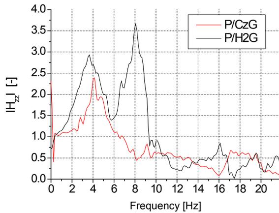
Fig. 11. Absolute acceleration transmittance values (floor-head): a comparison between P/CzG and P/H2G
