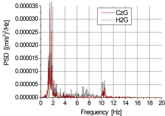
Fig. 9. Power spectral density values of head acceleration: a comparison between CzG and H2G
