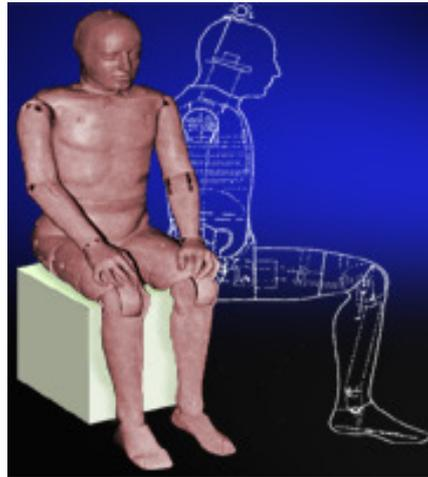
Fig. 2. Hybrid II 50<sup>th</sup> percentile male dummy [3]
