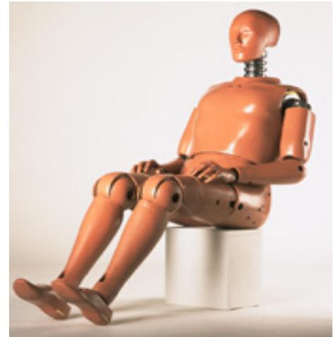
Fig. 3. Example test dummy of new generation: a 95<sup>th</sup> percentile male dummy of the Hybrid III family [4]
