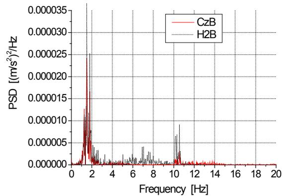
Fig. 10. Power spectral density values of thorax acceleration: a comparison between CzB and H2B
