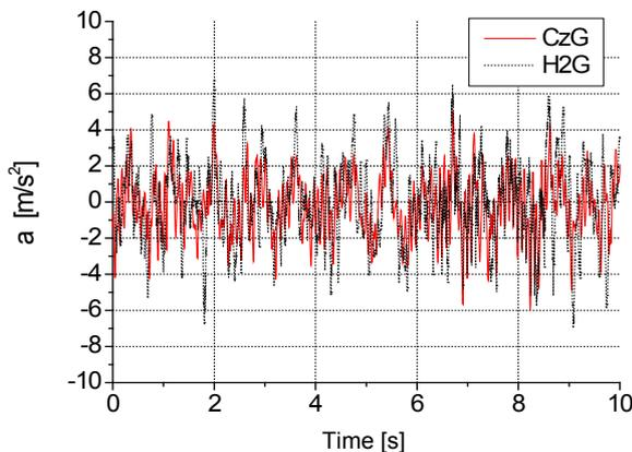
Fig. 7. Head acceleration vs. time curves: a comparison between CzG and H2G
