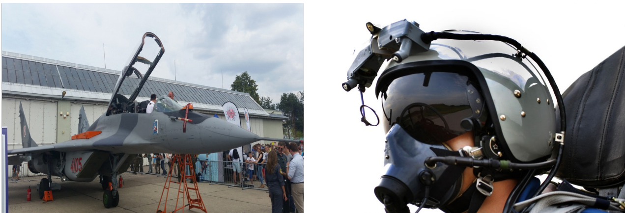
Fig. 5. View of the MiG-29 aircraft (left) and the SzCz-3 helmet-mounted imaging and communication system (right)
