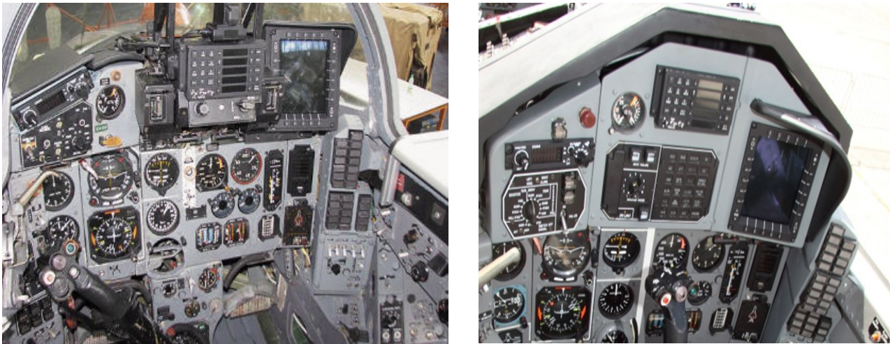
Fig. 2. View of the MiG-29 aircraft cabin after installation of an integrated avionics system by WZL-2 S.A.
