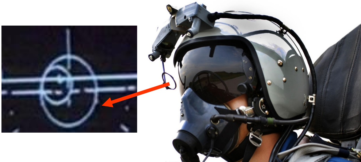
Fig. 4. View of the helmet with the SzCz-3UM targeting system, imaging method
