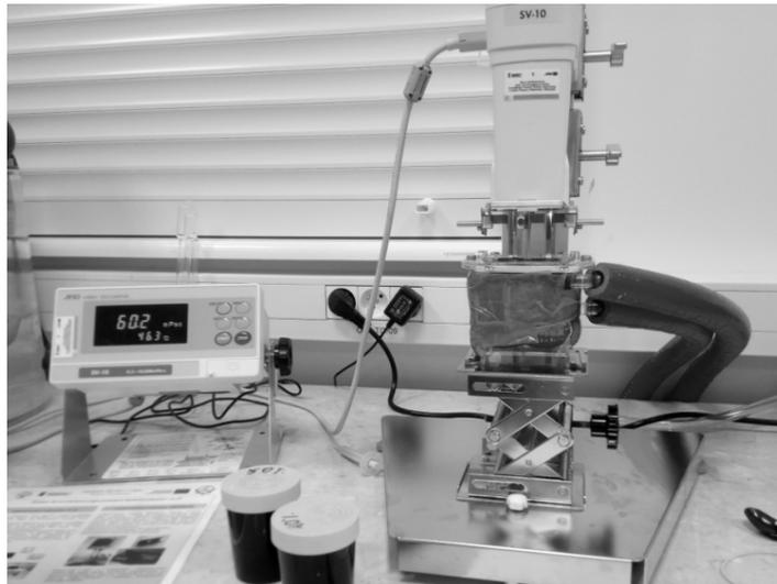
Fig. 1. The Vibro Viscometer SV 10
