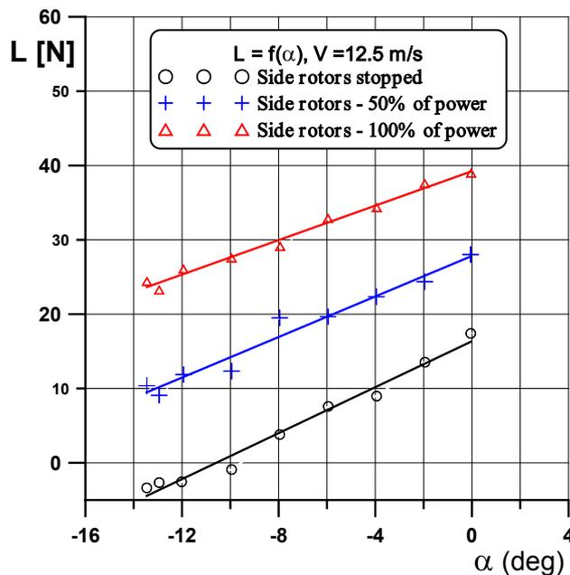
Fig. 6. Influence of the side rotors using 50% and 100% of their engine power on the autogyro lift
