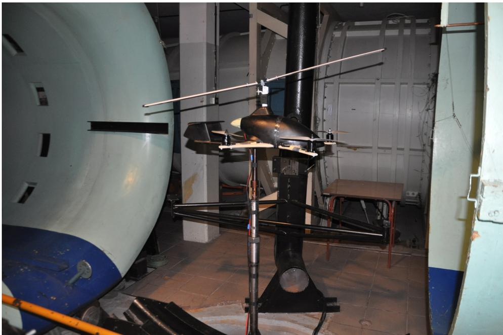
Fig. 3. The model of autogyro fixed to the wind tunnel model base
