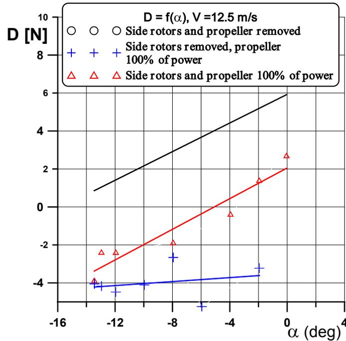
Fig. 7. Influence of the side rotors and propeller on the autogyro drag
