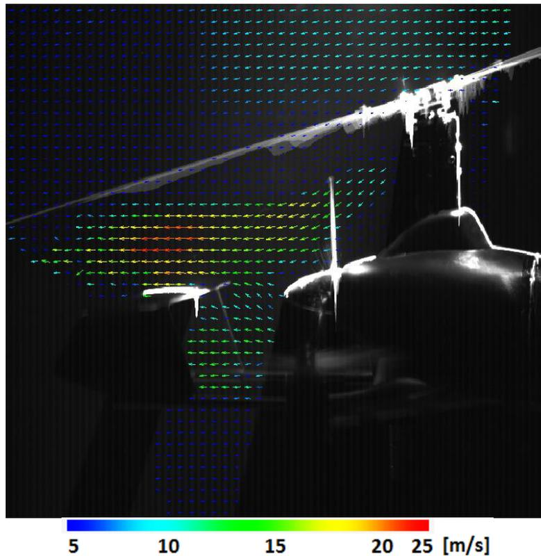
Fig. 9. PIV image depicting vector velocity field for side rotors and propeller working at 100% of their power and  $\Theta = 12.5^\circ$ ,  $V_\infty = 13.5$  m/s,  $\alpha = 0^\circ$
