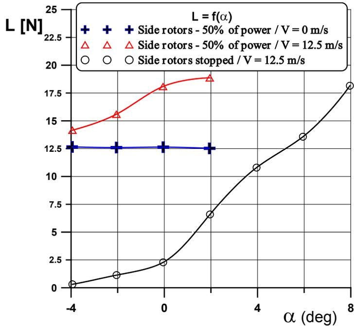
Fig. 5. Influence of the side rotors using 50% of their engine power on the autogyro lift
