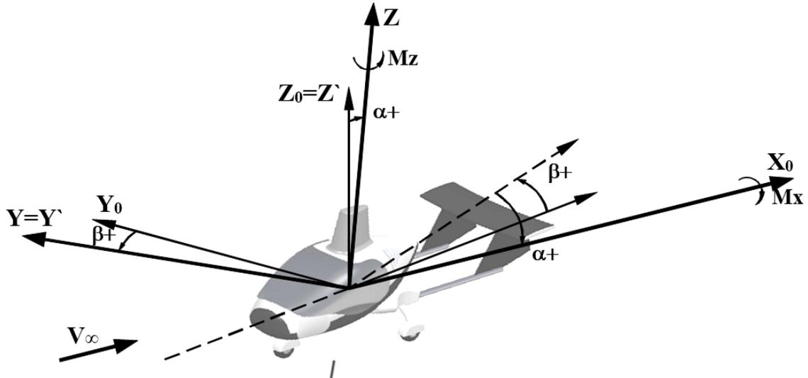
Fig. 4. The used coordinate system
