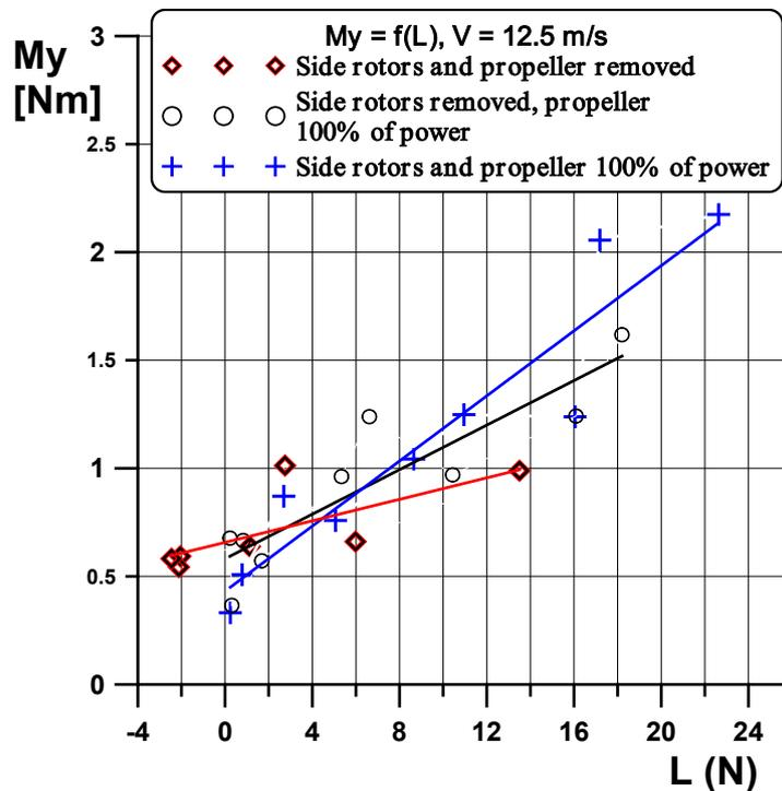
Fig. 8. Influence of the side rotors and propeller on the autogyro pitching moment
