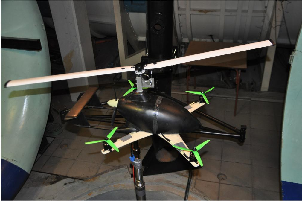
Fig. 2. The model of autogyro in T-1 IoA wind tunnel
