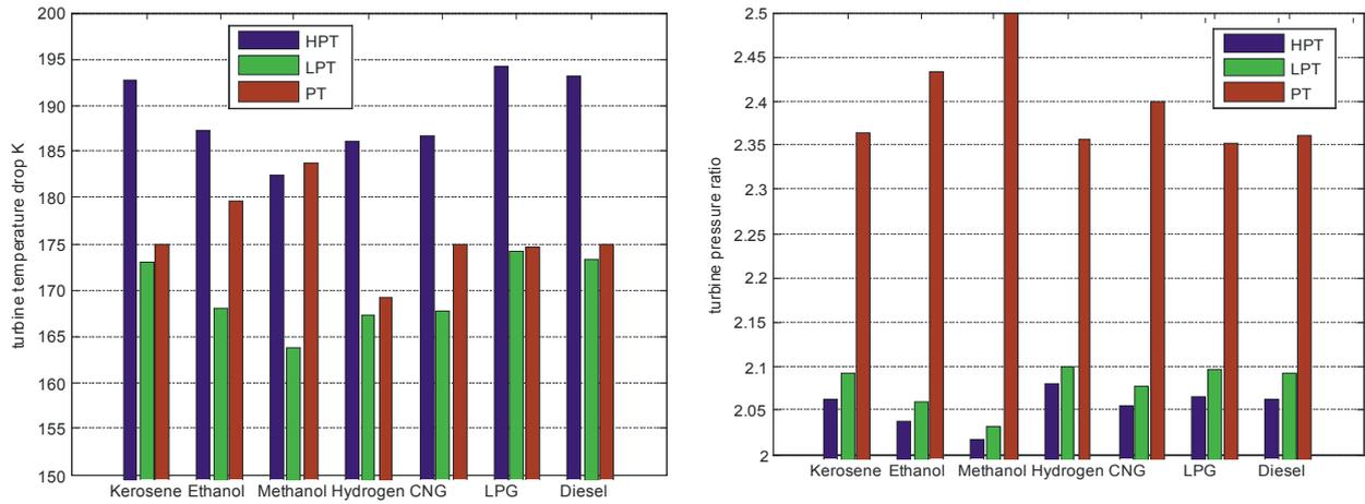
Fig. 2. Temperature drop and turbines pressure ratio of the engine fuelled by some kind of fuel (HPT – high-pressure turbine, LPT – low-pressure turbine, PT – power turbine)
