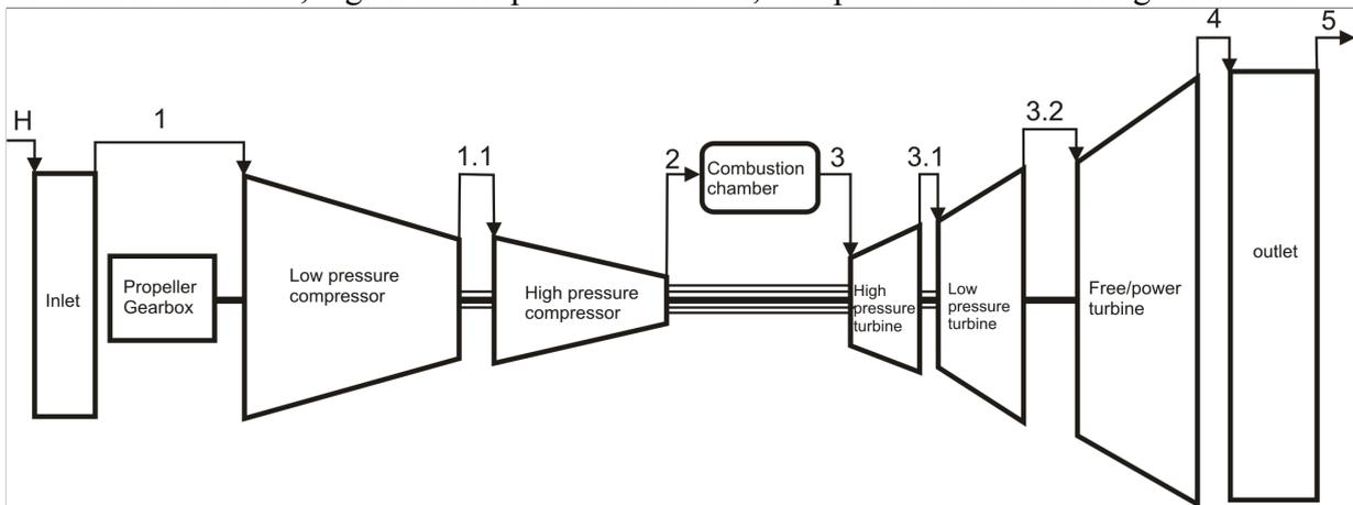
Fig 1. Three spool turboprop engine main components
