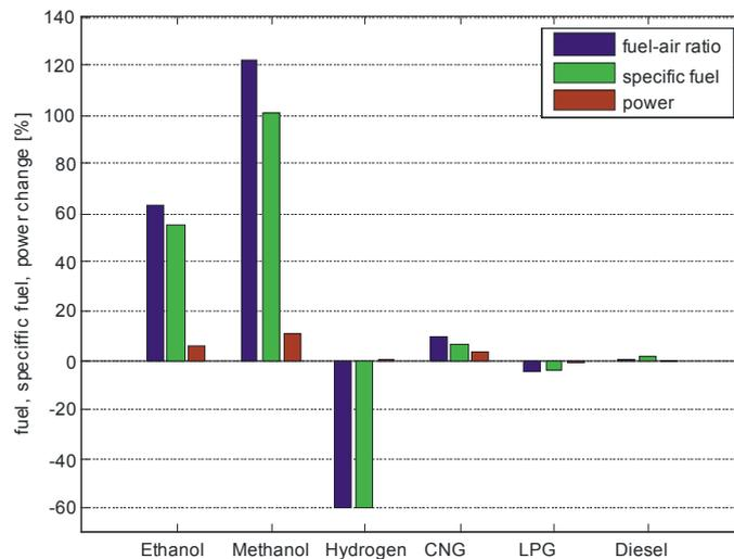
Fig. 1. Engine fuel consumption, specific fuel consumption and power for various fuels change into the engine fuelled by kerosene
