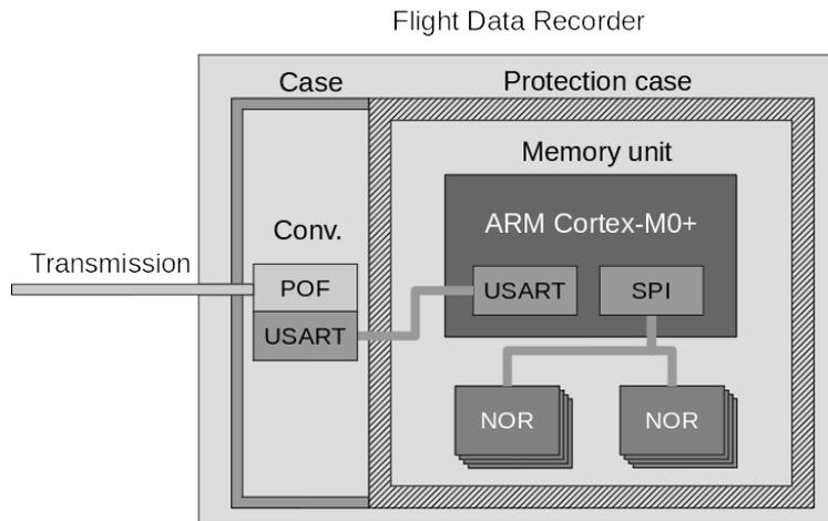
Fig. 2. Flight Data Recorder conception
