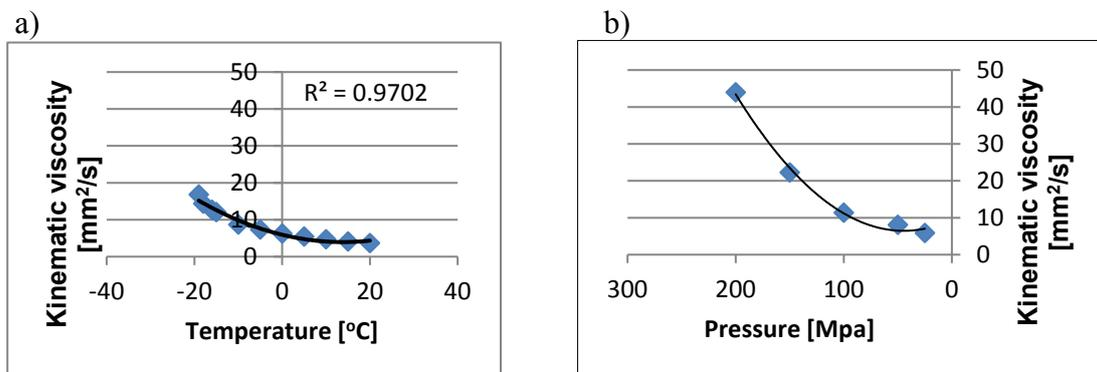
Fig. 3. The mineral diesel fuels viscosity change a) by cooling and b) by increase of the pressure
