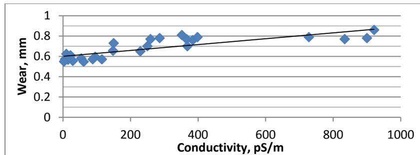
Fig. 7. Relationship between wear after BOCLE test obtained for the number of Jet fuel blends with synthetic hydrocarbons and alcohols and conductivity of these blends
