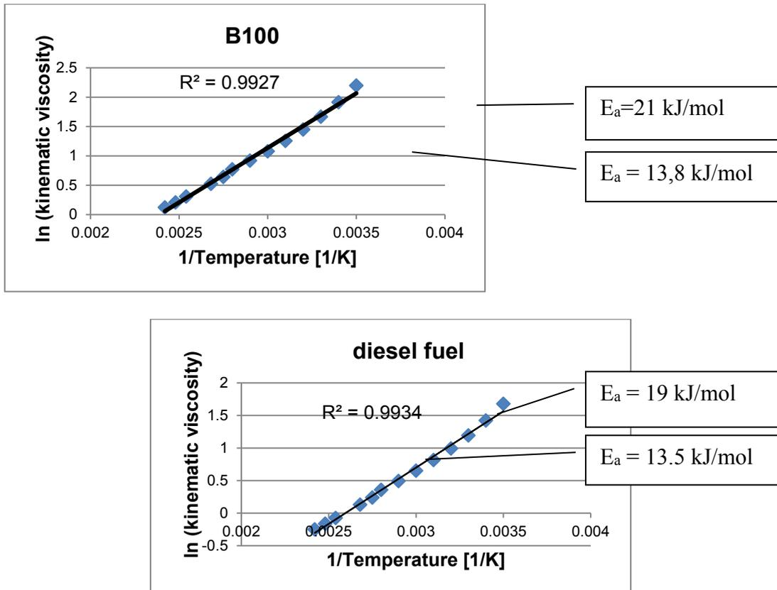
Fig. 2. Activation energy  $E_a$  of disruption reaction of intermolecular bonds, calculated for FAME (B100) and diesel fuel
