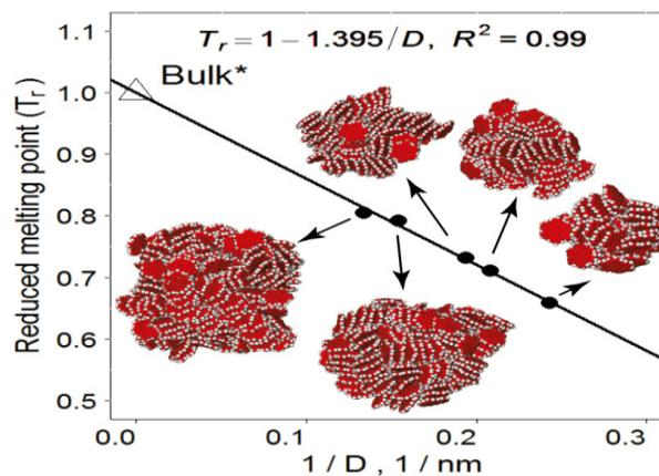
Fig. 4. Relation between reduced melting point and diameter of the clusters of PAH [4]
