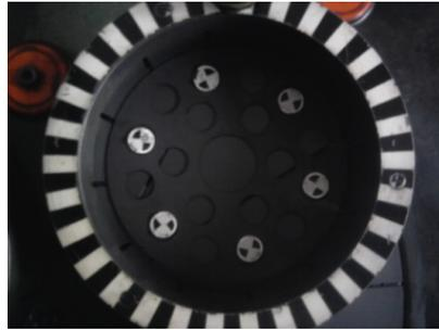
Fig. 4. Valve sealing lapped during the tests
