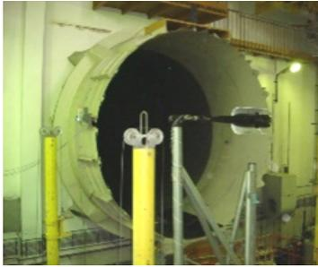
Fig. 3. The Sokol helicopter model with the passive armour model in the wind tunnel
