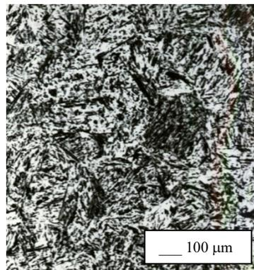
Fig. 8. Martensite (approx. 70%) in weld after welding with microjet cooling (air as microjet gas)
