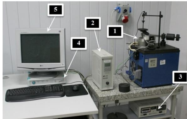
Fig. 2. Schema of the T-11 position for the tribological pin-on-disc-type test: 1 – sensors and transducers, 2 – the controller BT-11, 3 – the controller BT-03, 4 – digital amplifier 8 Spider, 5 – a set of computer
