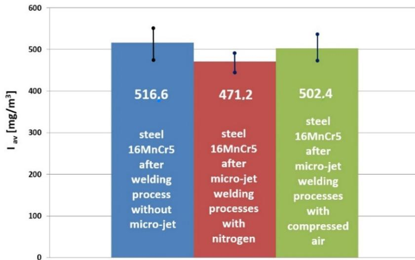
Fig. 12. Compilation of results for steel after welding process with micro-jet cooling and without cooling
