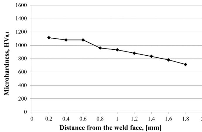
Fig. 9. Hardness of standard weld without micro-jet
