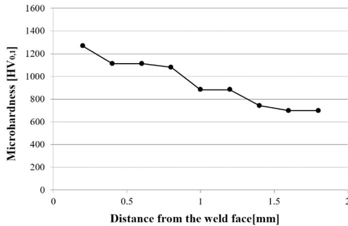
Fig. 11. Hardness of weld after micro-jet cooling, one cooling jet, air as a micro-jet gas
