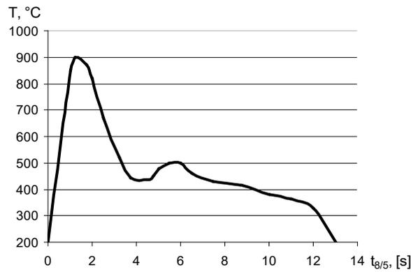
Fig. 5. Weld cooling conditions with micro-jet cooling, micro-jet gas (N<sub>2</sub>) pressure is 0.4 MPa, one jet installed in injector
