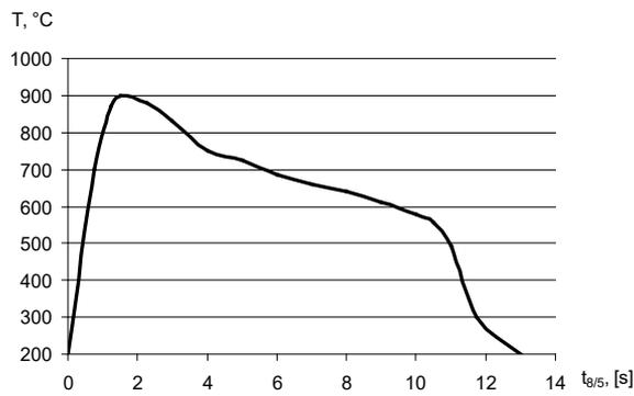
Fig. 6. Weld cooling conditions without micro-jet cooling
