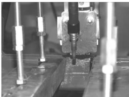
Fig. 1. Equipment for MIG welding with micro-jet injector (main view)
