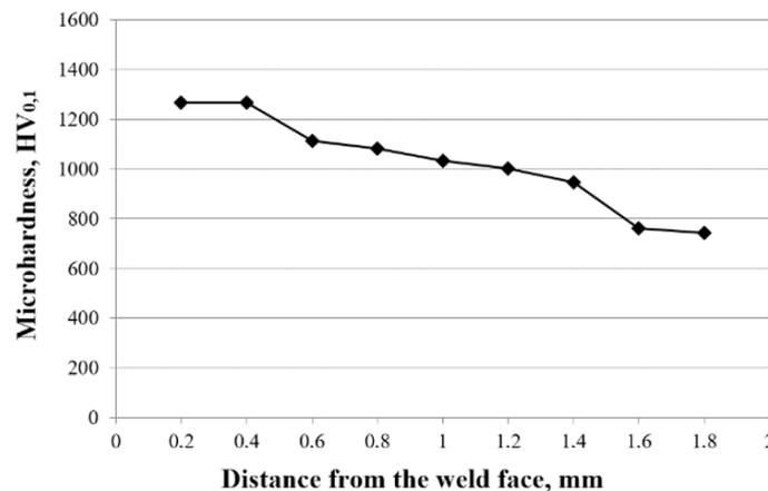
Fig. 10. Hardness of weld after micro-jet cooling, one cooling jet, nitrogen as a micro-jet gas
