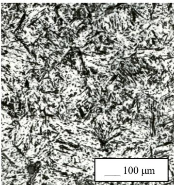
Fig. 7. Martensite (approx. 75%) in weld after welding with microjet cooling (nitrogen as microjet gas)
