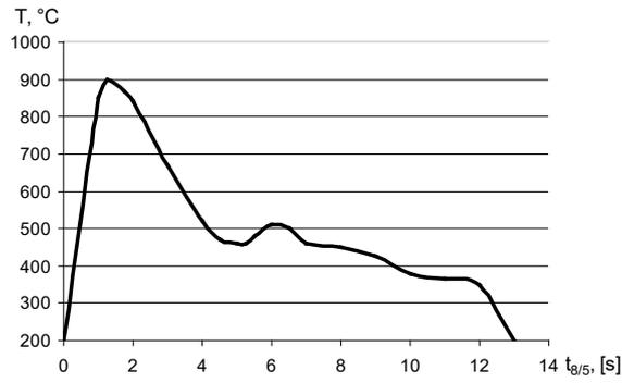
Fig. 4. Weld cooling conditions with micro-jet cooling, micro-jet gas (compressed air) pressure is 0.4 MPa, one jet installed in injector
