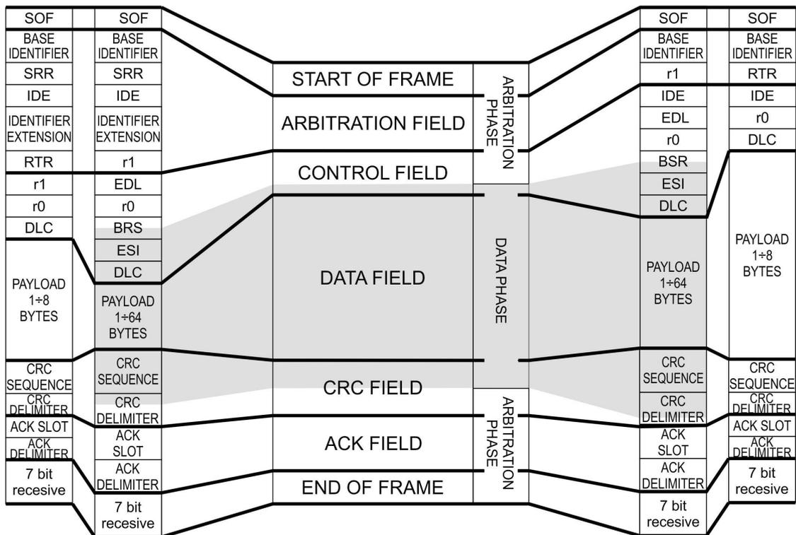
Fig. 5. The scheme of CAN-FD message frame
