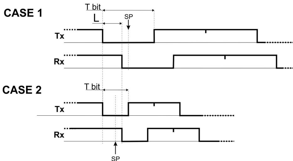
Fig. 4. The scheme of error caused by to high bandwidth
