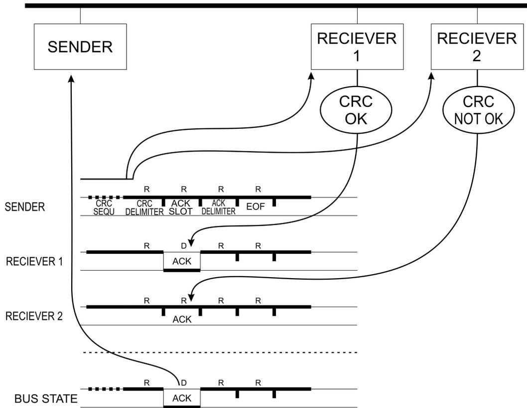
Fig. 3. CAN acknowledge bit check
