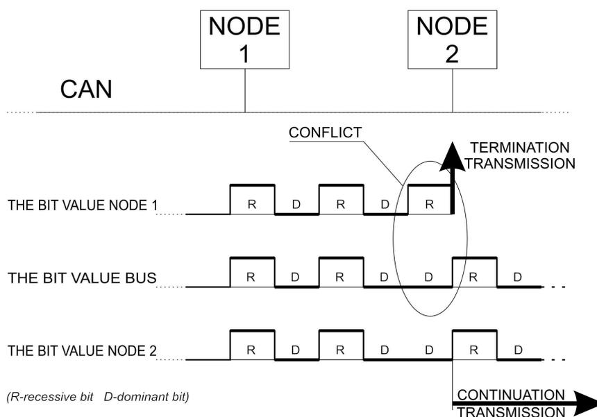
Fig. 1. example of CAN arbitration
