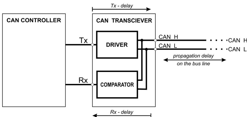
Fig. 2. Scheme of CAN transceiver
