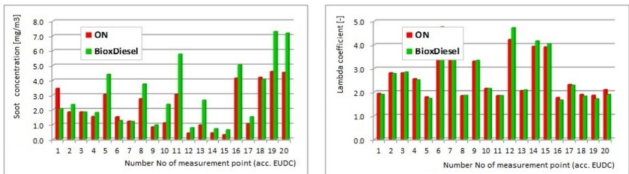
Fig. 7. Results of emission testing of 1.3 SDE engine: soot and lambda coefficient
