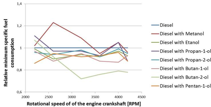
Fig. 10. Relative specific fuel consumption generated by the engine fed with mixtures of Diesel and heavier alcohol
