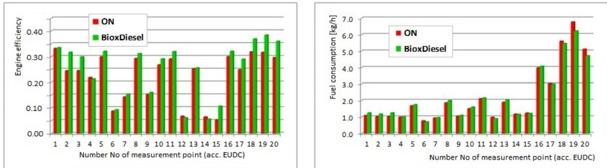
Fig. 5. Results of the performance testing of the 1.3 SDE Diesel engine: engine efficiency, fuel consumption
