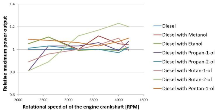
Fig. 8. Power generated by the engine fed with mixtures of Diesel and heavier alcohol
