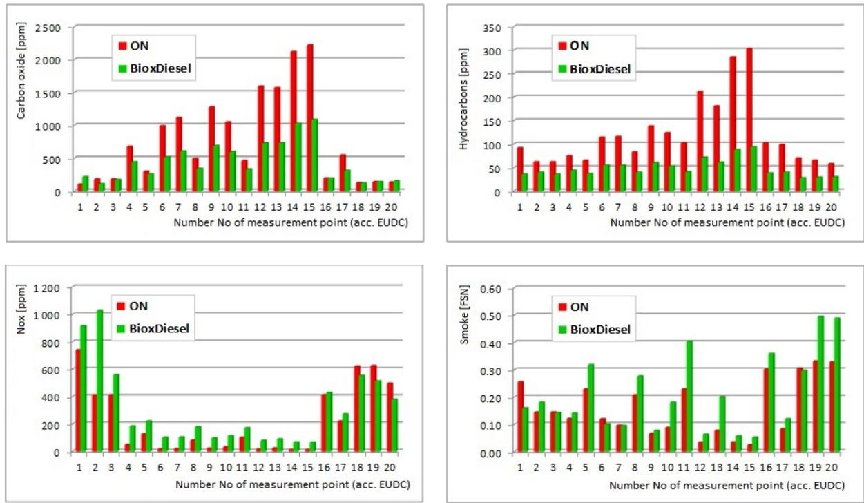
Fig. 6. Results of emission testing of 1.3 SDE engine: carbon oxide, hydrocarbons, nitrogen oxides and smoke
