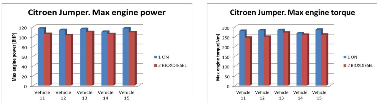
Fig. 2. Comparison of measured power and torque generated by the engine for two different fuels Citroen Jumper parcel delivery vans. Measurement taken on the first day of testing on the vehicle test bed
