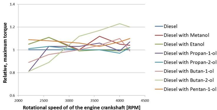
Fig. 9. Torque generated by the engine fed with mixtures of Diesel and heavier alcohol
