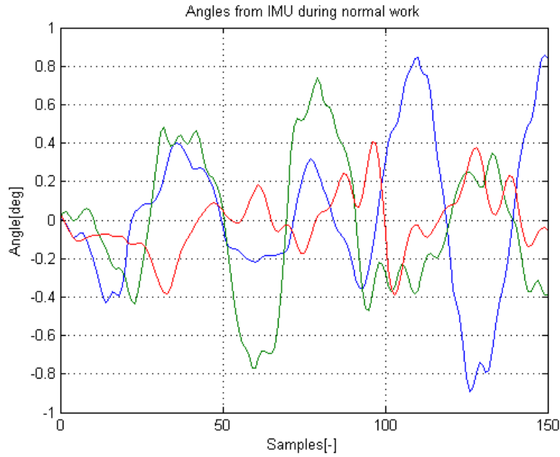
Fig. 1. Pitch, Roll, Yaw angle during normal work of optoelectronic head
