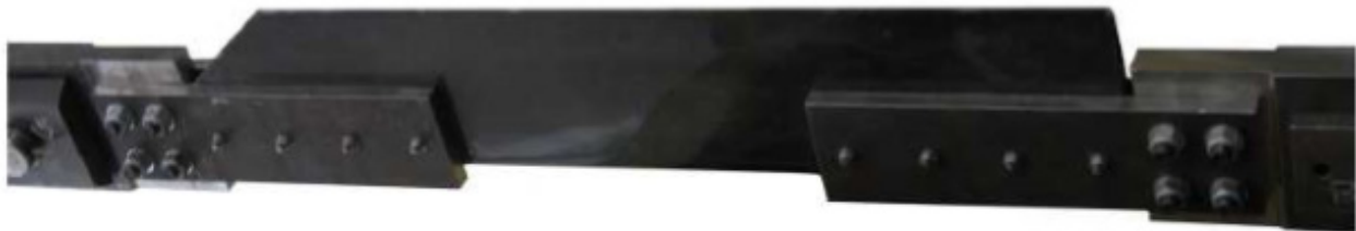
Fig. 2. Strength test object with elements to introduction load
