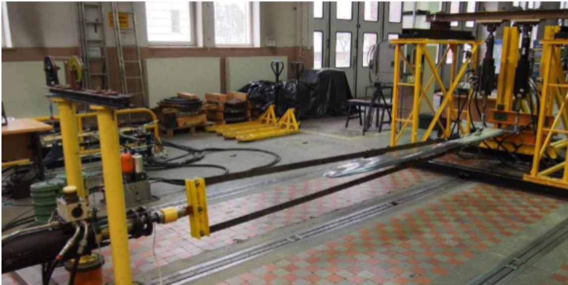
Fig. 11. Test stand of delamination study
