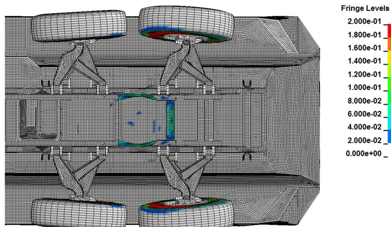
Fig. 5. Plastic strain of the element of the construction of the underbody resulting from non-contact explosion
