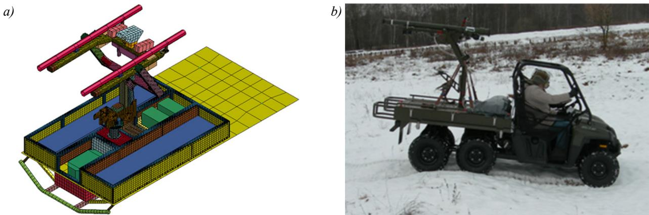
Fig. 8. „Kusza” anti-aircraft weapon system: a) model, b) anti-aircraft launcher on Polaris Ranger 6x6 underbody during training ground tests under winter conditions
