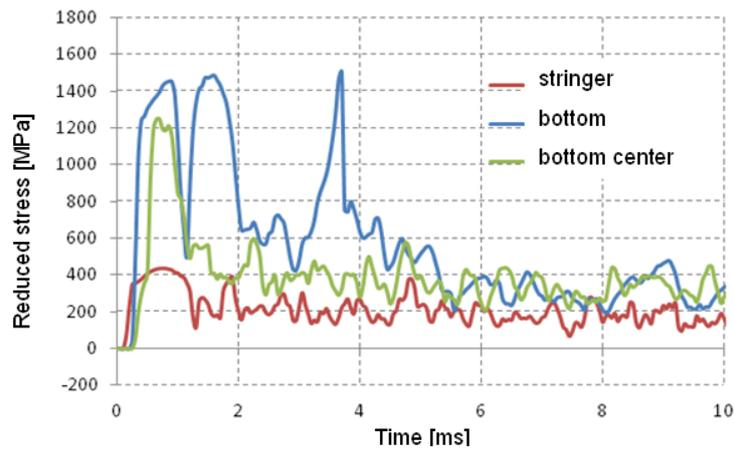
Fig. 4. Changes in tensions in selected structural nodes resulting from non-contact explosion
