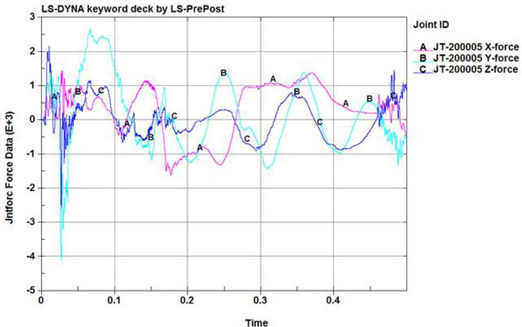
Fig. 9. Change of forces over time at the joint of the load-bearing structure of the anti-aircraft launcher
