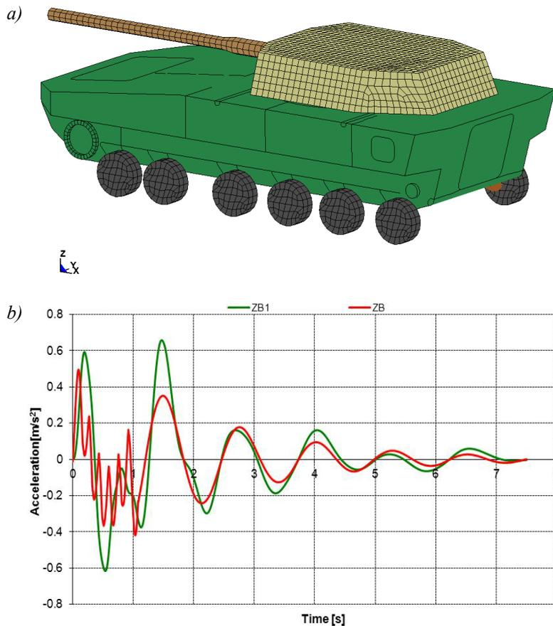
Fig. 7. Direct Fire Support Vehicle: a) model, b) vertical accelerations acting on the vehicle and its crew while travelling through a single obstacle
