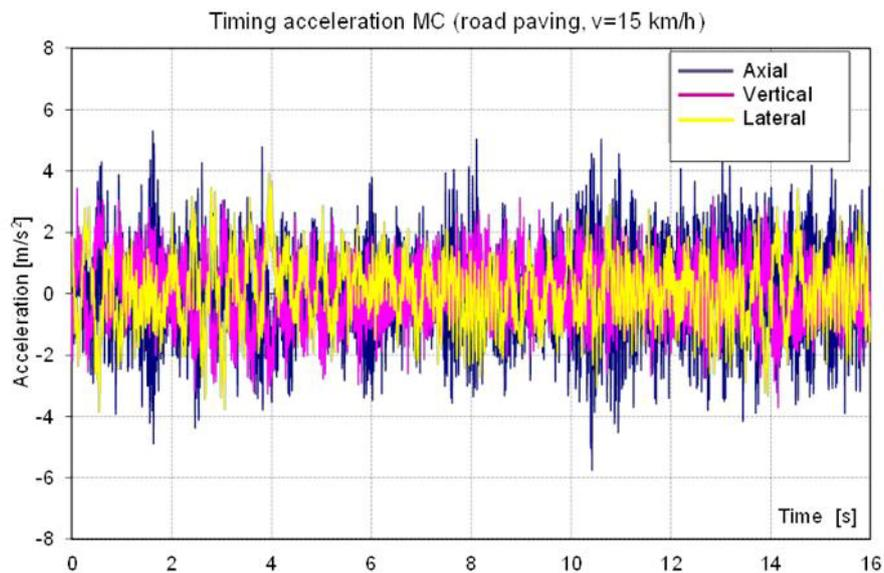
Fig. 2. Accelerations acting on the centre of mass of the tank over time during the travel with  $v = 15 \text{ km/h}$
