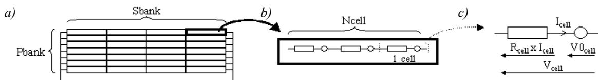
Fig. 5. Example of battery in AMESim, a) source of current consist of accumulators connected in series and parallel, b) battery consist of 3 cells, c) equivalent circuit of the cell, where  $I_{cell}$  – cell current;  $V_{cell}$  – cell voltage [1]
