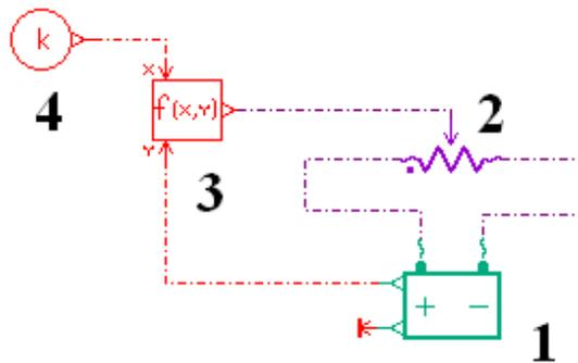
Fig. 3. Test stand modelled in AMESim software: 1 – battery, 2 – resistor, 3 – current loop, 4 – current set value
