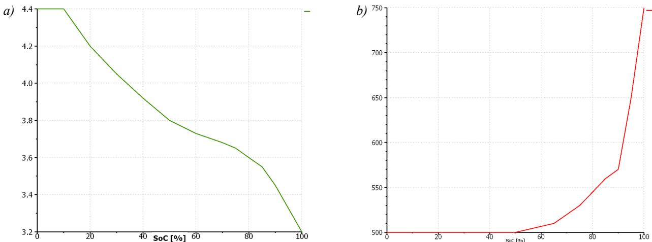
Fig. 4. KOKAM SLPB 120216216 cell state of charge modelled in AMESim software: a) voltage of battery, b) internal resistance of the cell
