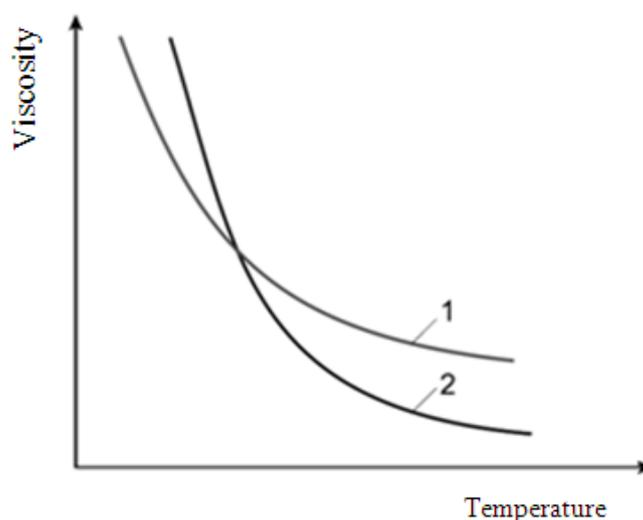
Fig. 1. An example of graph of viscosity-temperature changes; 1 – oil with a low viscosity variation of temperature, 2 – oil with a high viscosity variation of temperature [18]
