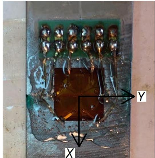
Fig. 4. Orientation of strain gauge rosette
