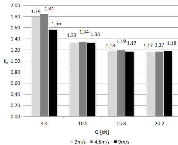
Fig. 7. Dynamic factors for braking of the drive system with the lead screw for various load and carriage speed
