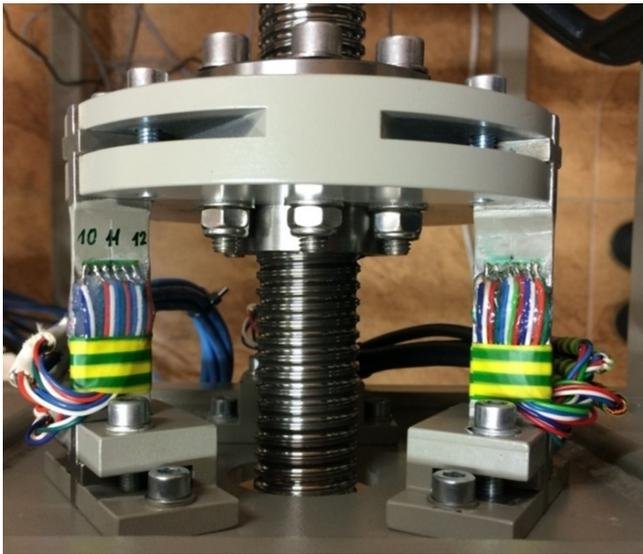
Fig. 3. Nut bracket for strain gauge measurements of axial force and torque on a nut of the lead screw
