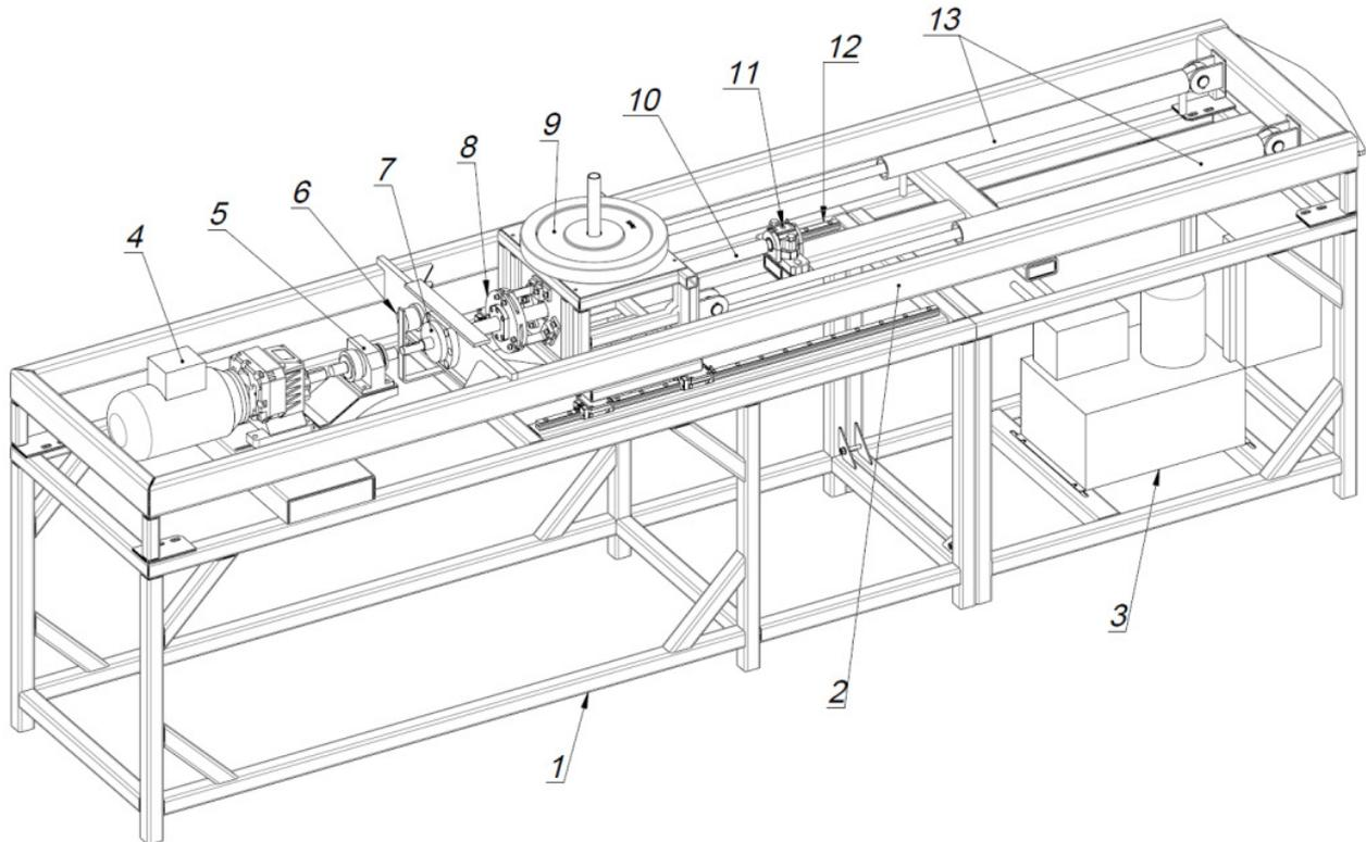
*Fig. 1. A concept of the test stand for lead screws*
