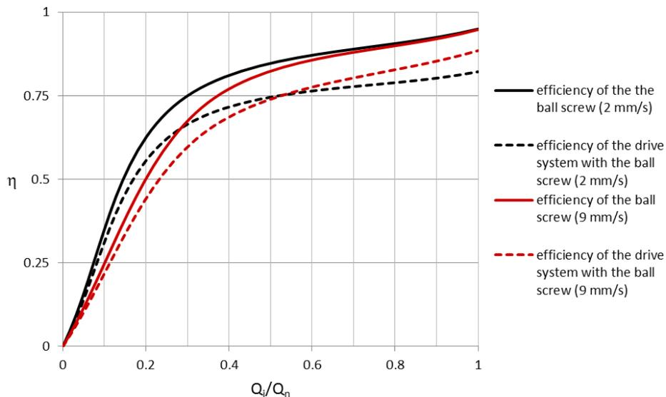
Fig. 5. The efficiency of the drive system and the lead screw
