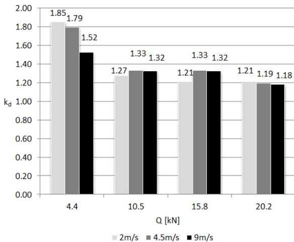
Fig. 6. Dynamic factors for start-up of the drive system with the lead screw for various load and carriage speed
