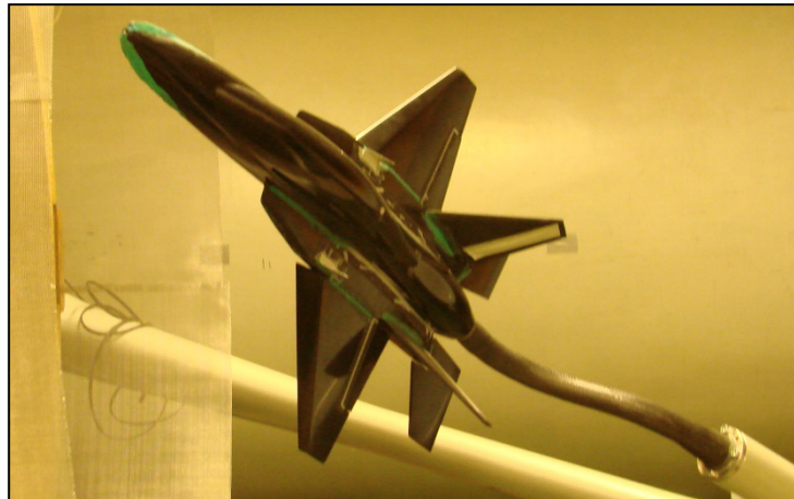
Fig. 6. Aerodynamic model in the test section of the low speed wind tunnel
