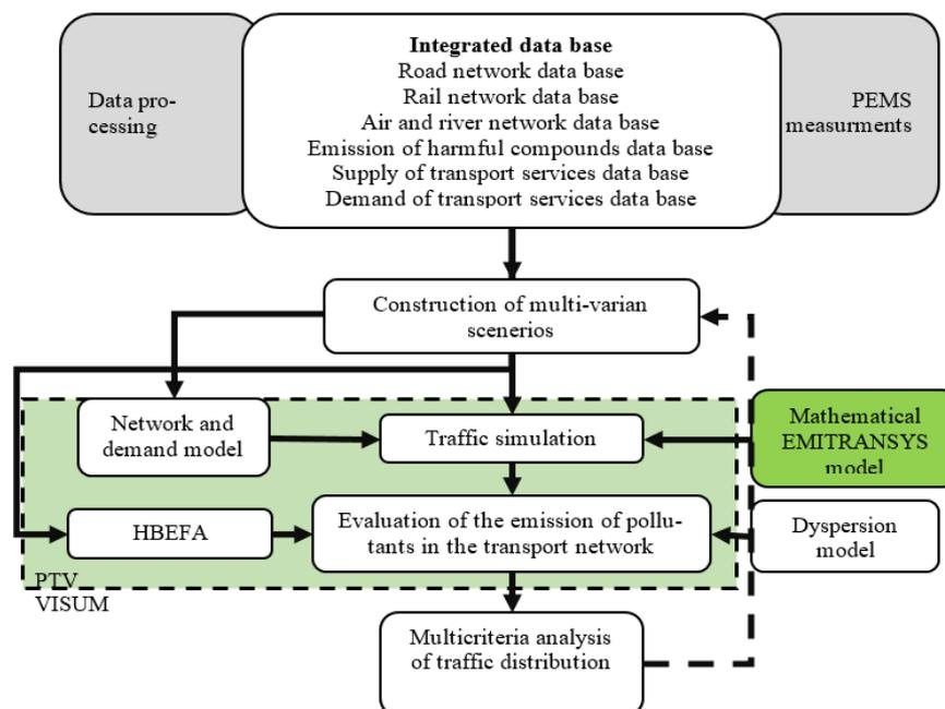
Fig. 2. EMITRANSYS model elements in VISUM
