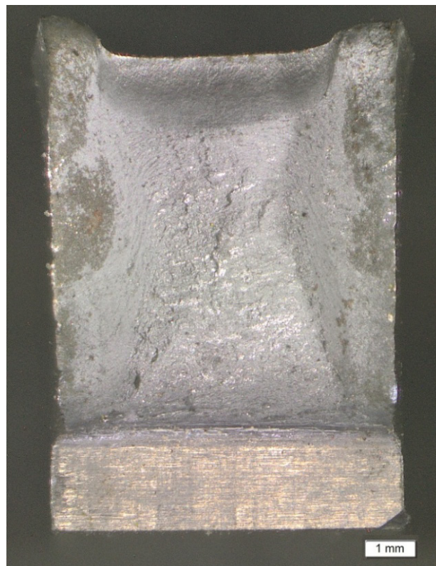
Fig. 5. View late sample notched in the weld
