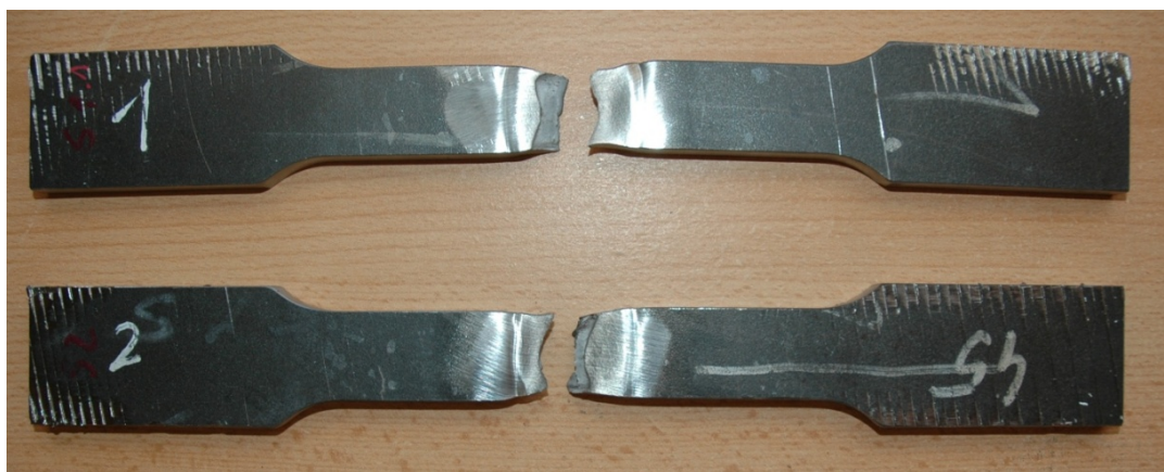
Fig. 3. View samples of welded joints of steel Weldox 1300 after tensile test
