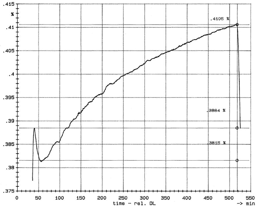
Fig. 12. Course of the relative elongation in function of time during ageing of composite alloy at the temperature of 200°C for the first stage
