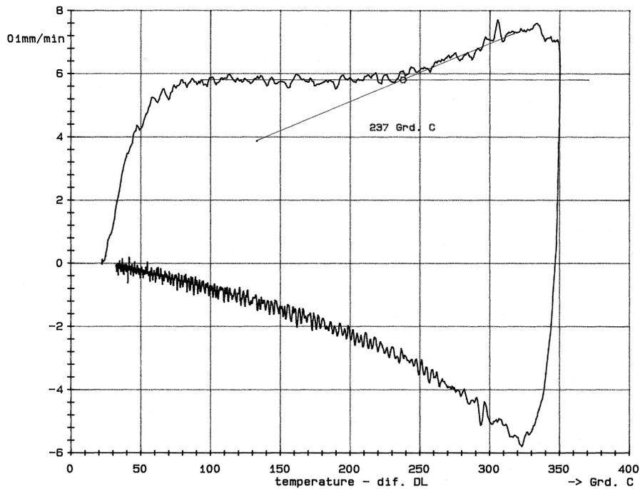
Fig. 9. Course of the derived function of the extension in relation to time  $dL/dt$  versus temperature for the standard alloy on pistons
