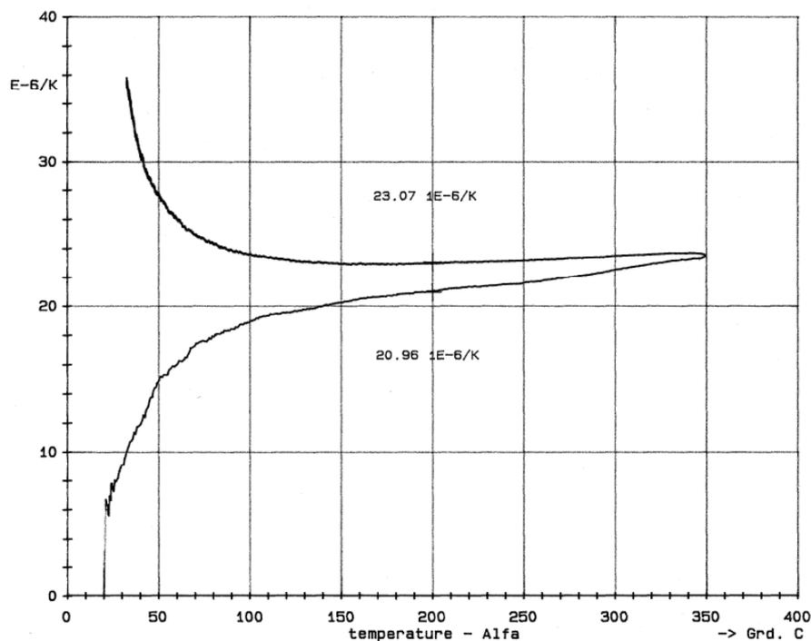
Fig. 5. Course of the coefficient of linear thermal expansion  $\alpha$  versus temperature during heating and cooling for the standard alloy
