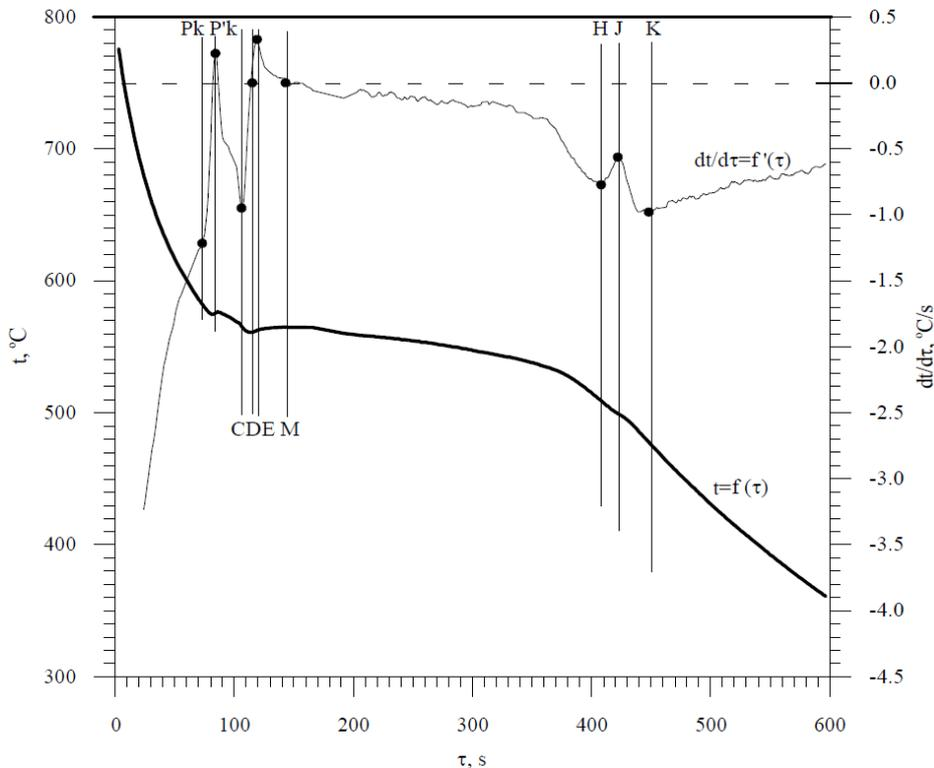
Fig. 2. ATD of novel composite alloy
