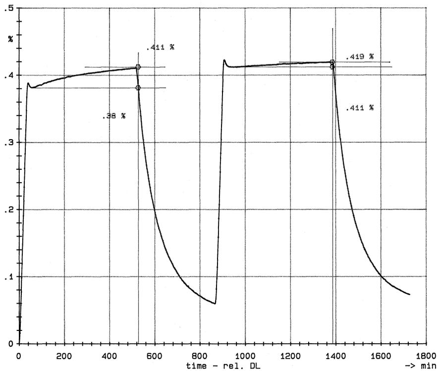
Fig. 11. Course of the relative elongation in function of time during ageing of composite alloy at the temperature of 200°C with two-stage ageing process
