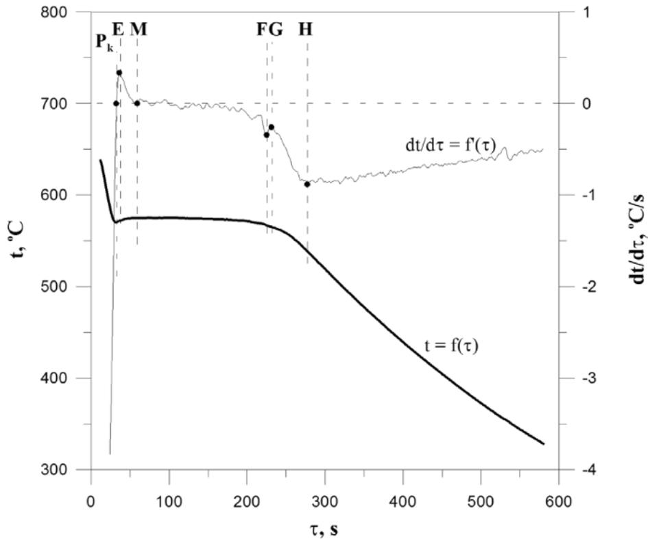
Fig. 1. ATD of standard alloy – silumin Ak12
