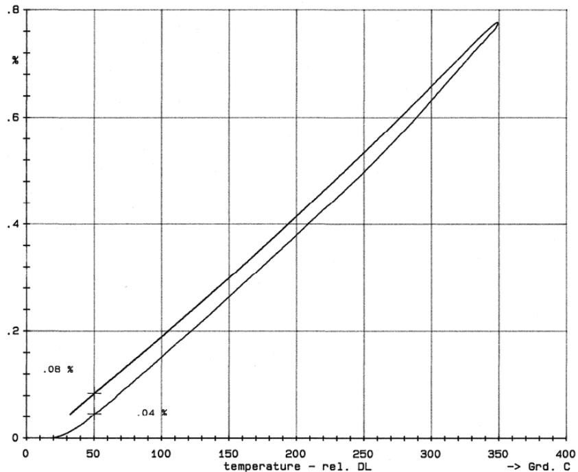
Fig. 7. Course of the relative piston elongation  $\Delta L/L_0$  versus temperature during heating and cooling for the standard alloy
