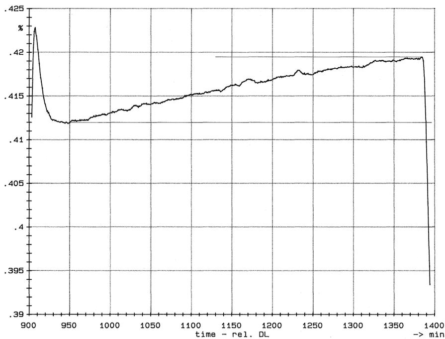
Fig. 13. Course of the relative elongation in function of time during ageing of composite alloy at the temperature of 200°C for the second stage
