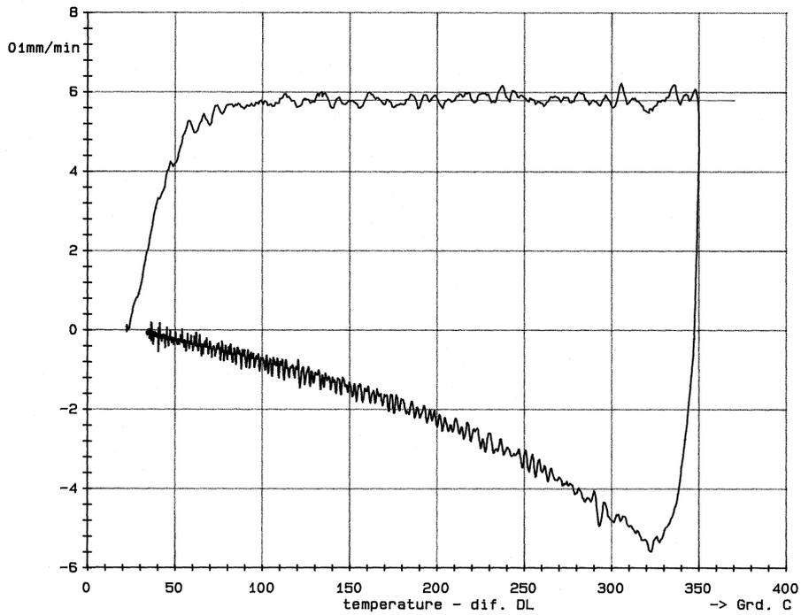
Fig. 10. Course of the derived function of the extension in relation to time  $dL/dt$  versus temperature during heating and cooling for the composite alloy on pistons
