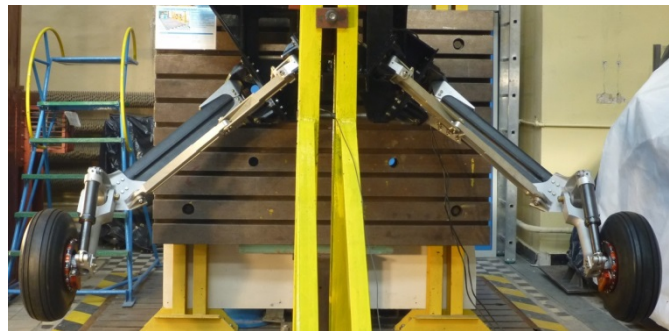
Fig. 3. AT-6 main landing gear: 1-composite leg, 2- main fitting, 3- upper fitting, 4- lever, 5-shock absorber, 6- wheel, 7- brake, 8- electro-actuator, 9- yoke, 10- drag strut (source: Institute of Aviation)
