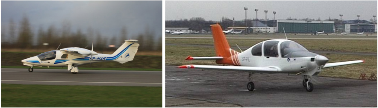
Fig. 1. Tricycle-type landing gear (EM-11C Orka and I23-Manager aircraft) [4]
