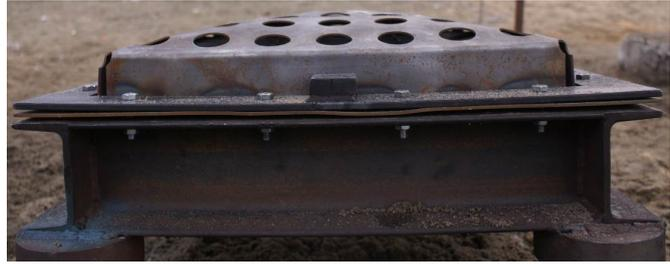
Fig. 7. The protective shield after the 0.75 kg TNT blast test: a) the isometric view, b) the front view
