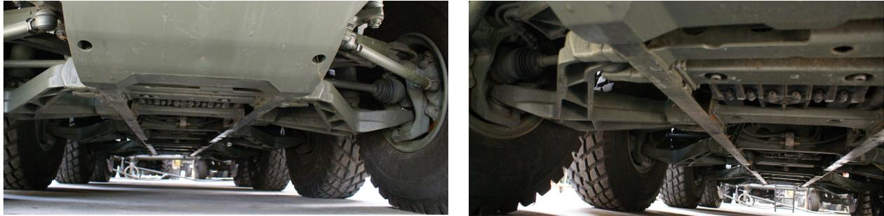
Fig. 1. Integrated bottom frame for the suspension and drive in the ROSOMAK-type LAV vehicle
