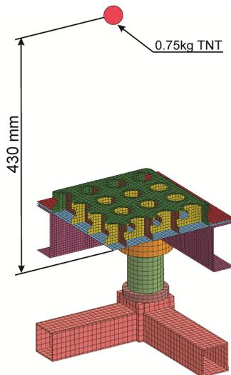
Fig. 5. Isometric view of the position of explosive charge in relation to the protection shield
