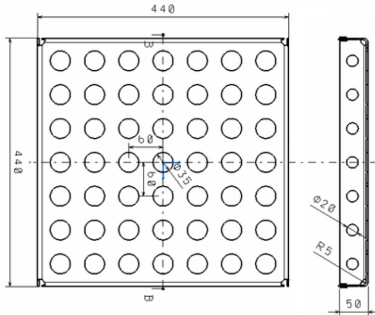
Fig. 3. Size of the protective shield
