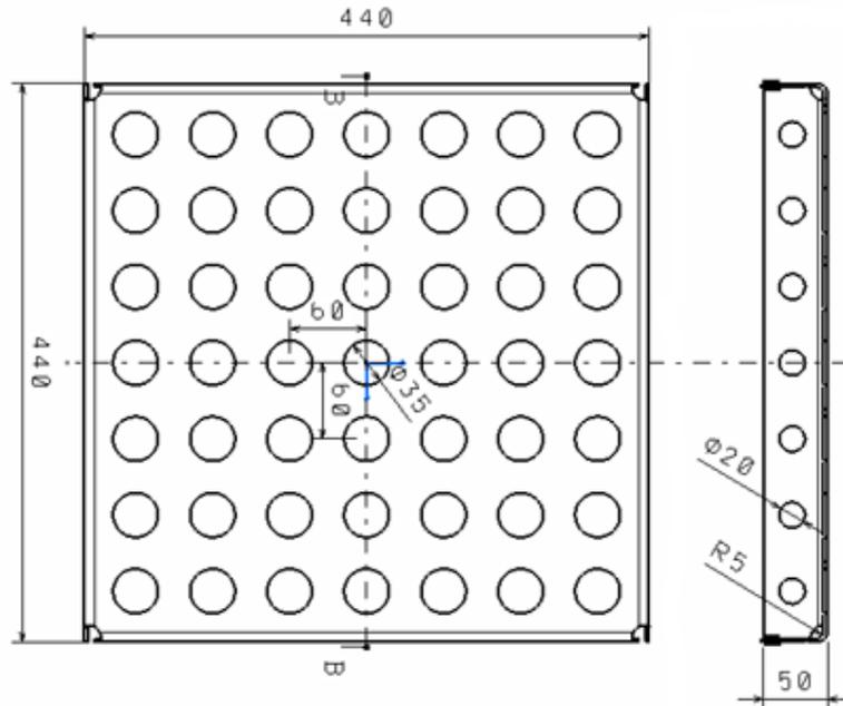
Fig. 3. Size of the protective shield
