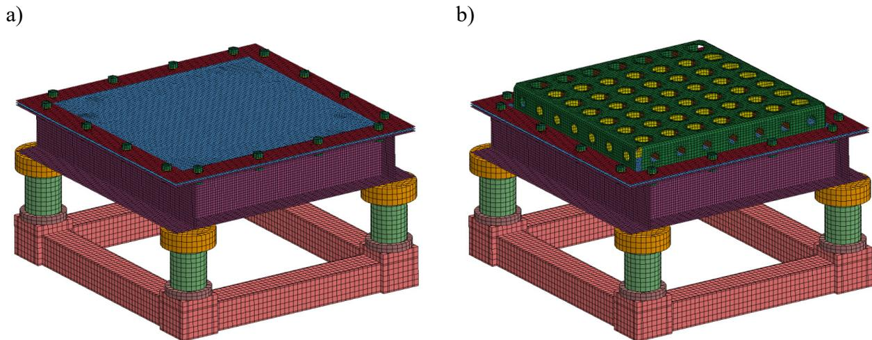
Fig. 4. Isometric view range stand with fixed panels for two variants a) reference system, b) system with the protective shield
