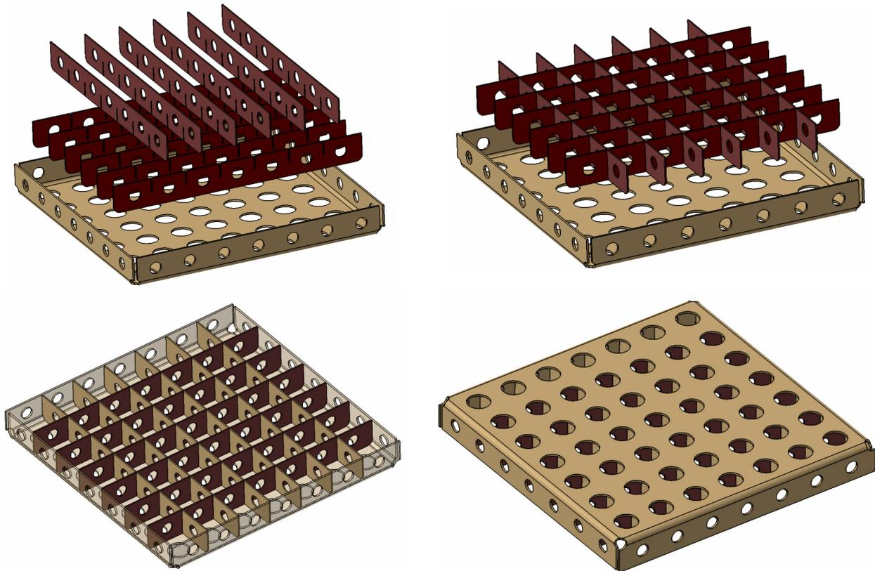
Fig. 2. Construction of the openwork steel shield
