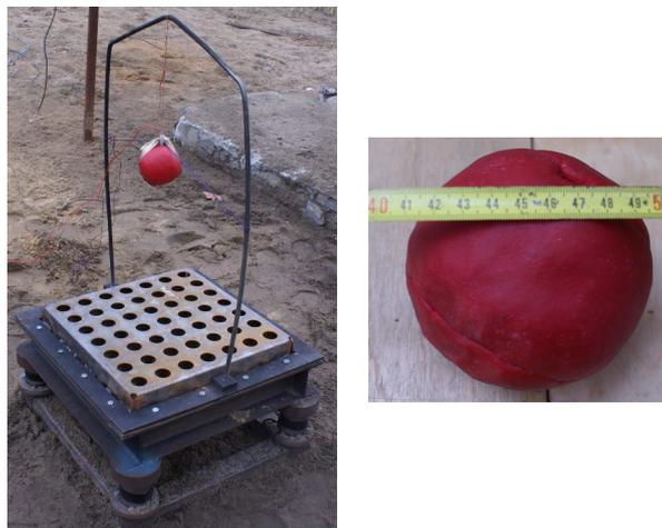
Fig. 6. The protective shield before the 0.75 kg TNT blast test
