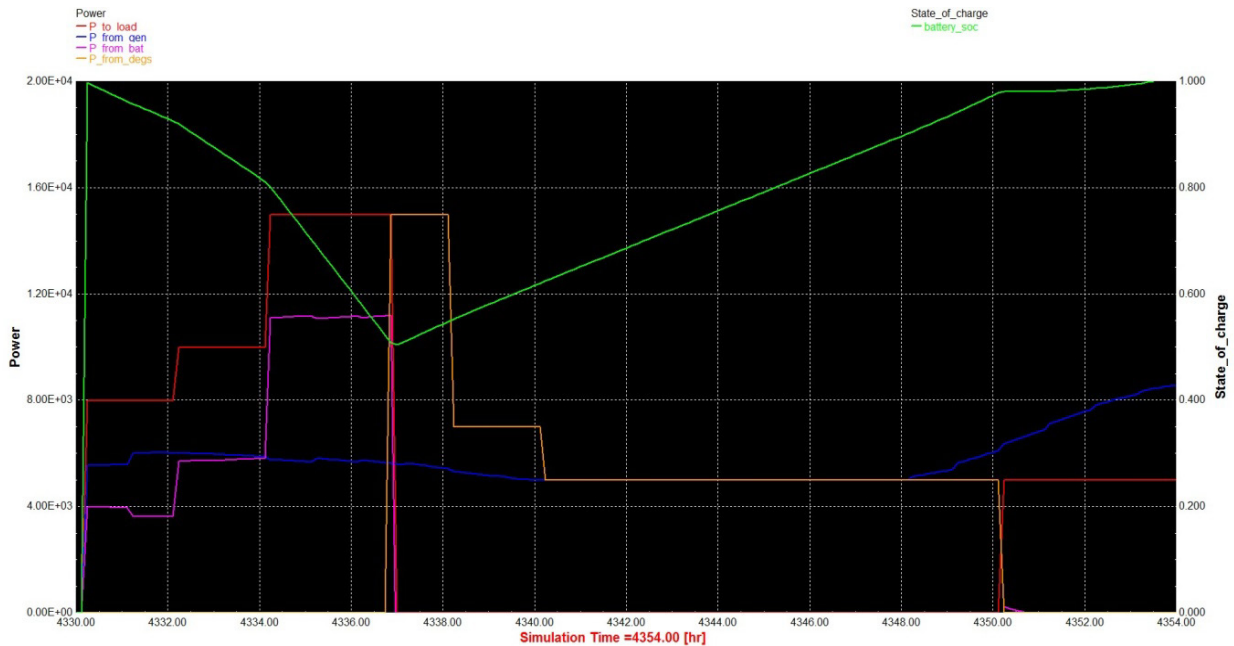
Fig. 4. System data from 24h simulation on 1 st of July in battery SOC based control scheme
