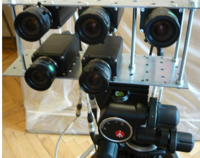
Fig. 2. The pentadruple GigE camera array – front view
