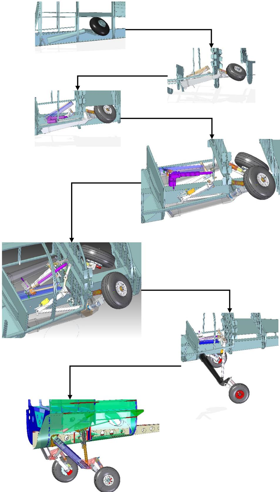
Fig. 1. The construction progress of landing gear
