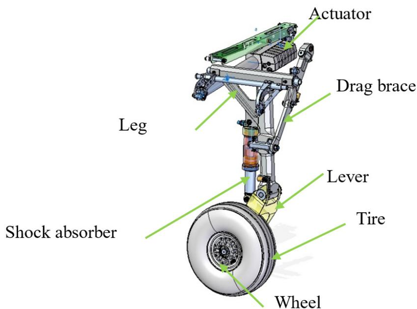
Fig. 2. The landing gear 3D model
