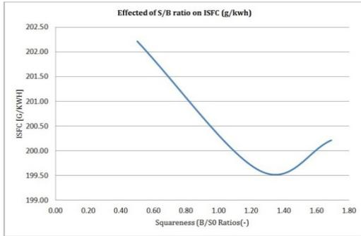
Fig 5(c). ISFC from AVL BOOST simulation
