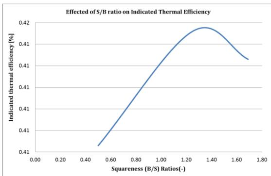
Fig. 4(a). Indicated thermal efficiency from AVL BOOST simulation
