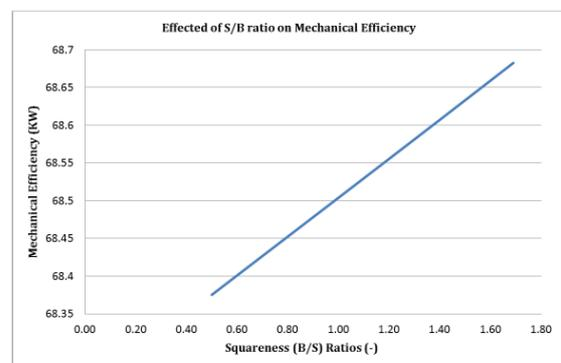
Fig. 4(b). Mechanical efficiency from AVL BOOST simulation
