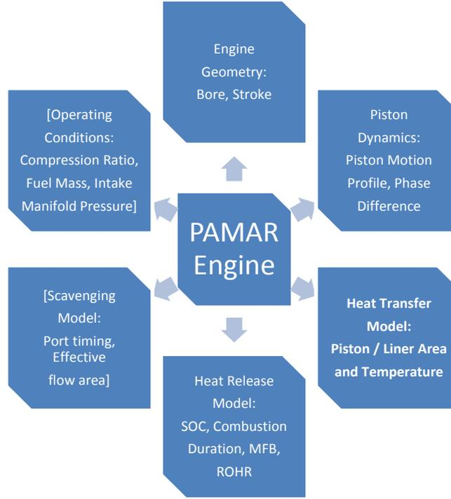
Fig. 1. Numerical model input data flow
