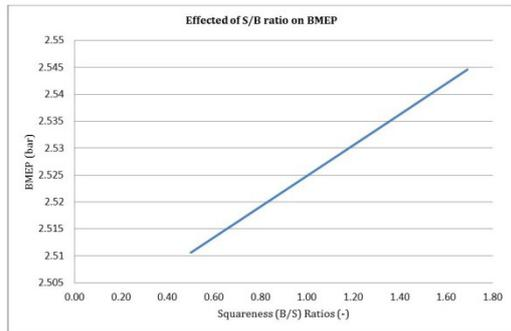
Fig 4(e). Brake Mean Effective Pressure from AVL BOOST simulation
