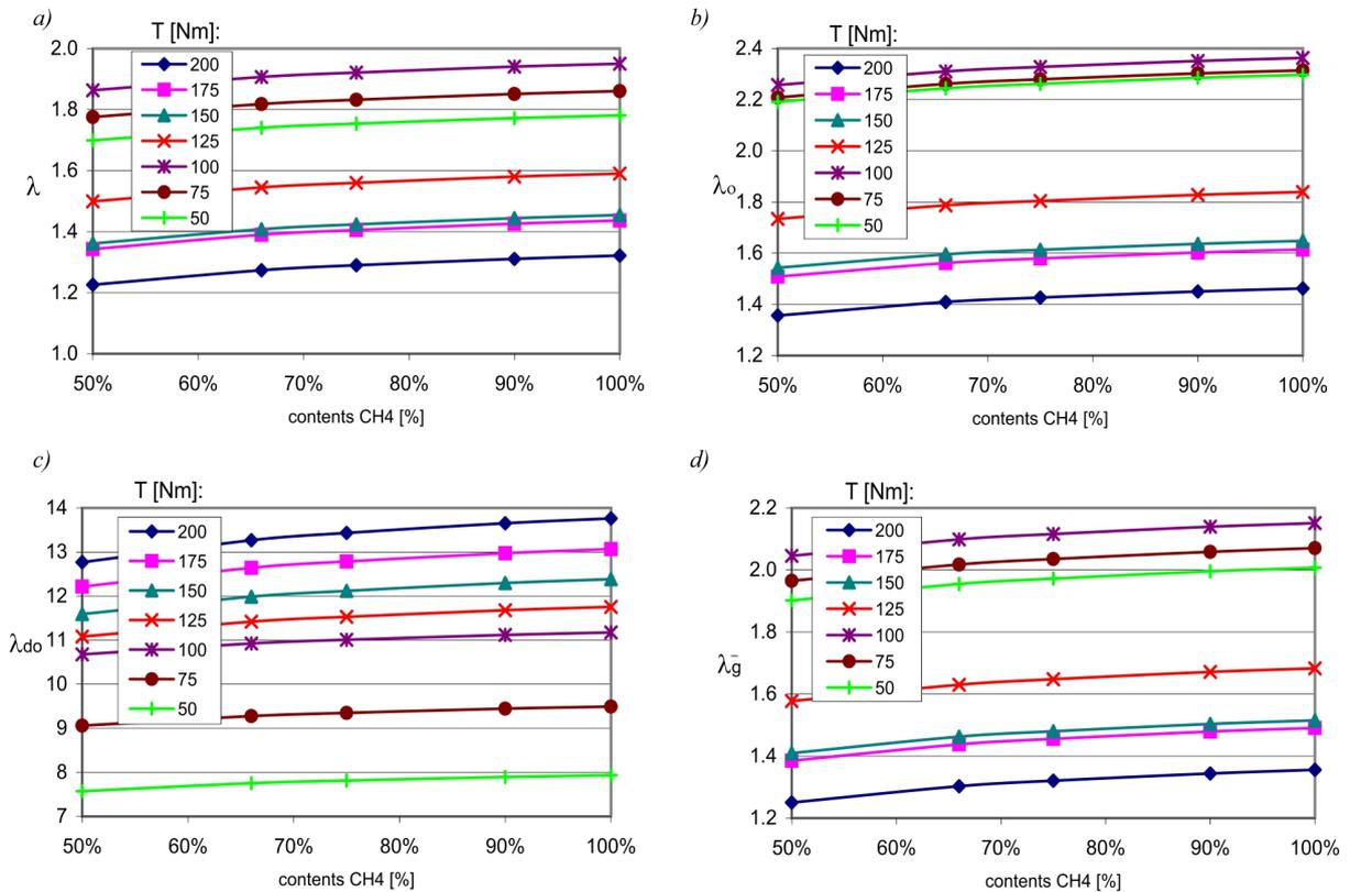
Fig. 5. The impact of the concentration of methane in biogas on the ratios characterising the mixture at  $n = 3000$  rpm with a 10% share of liquid fuel for various engine loads: a)  $\lambda$ , b)  $\lambda_o$  b)  $\lambda_{do}$  b)  $\lambda_g$
