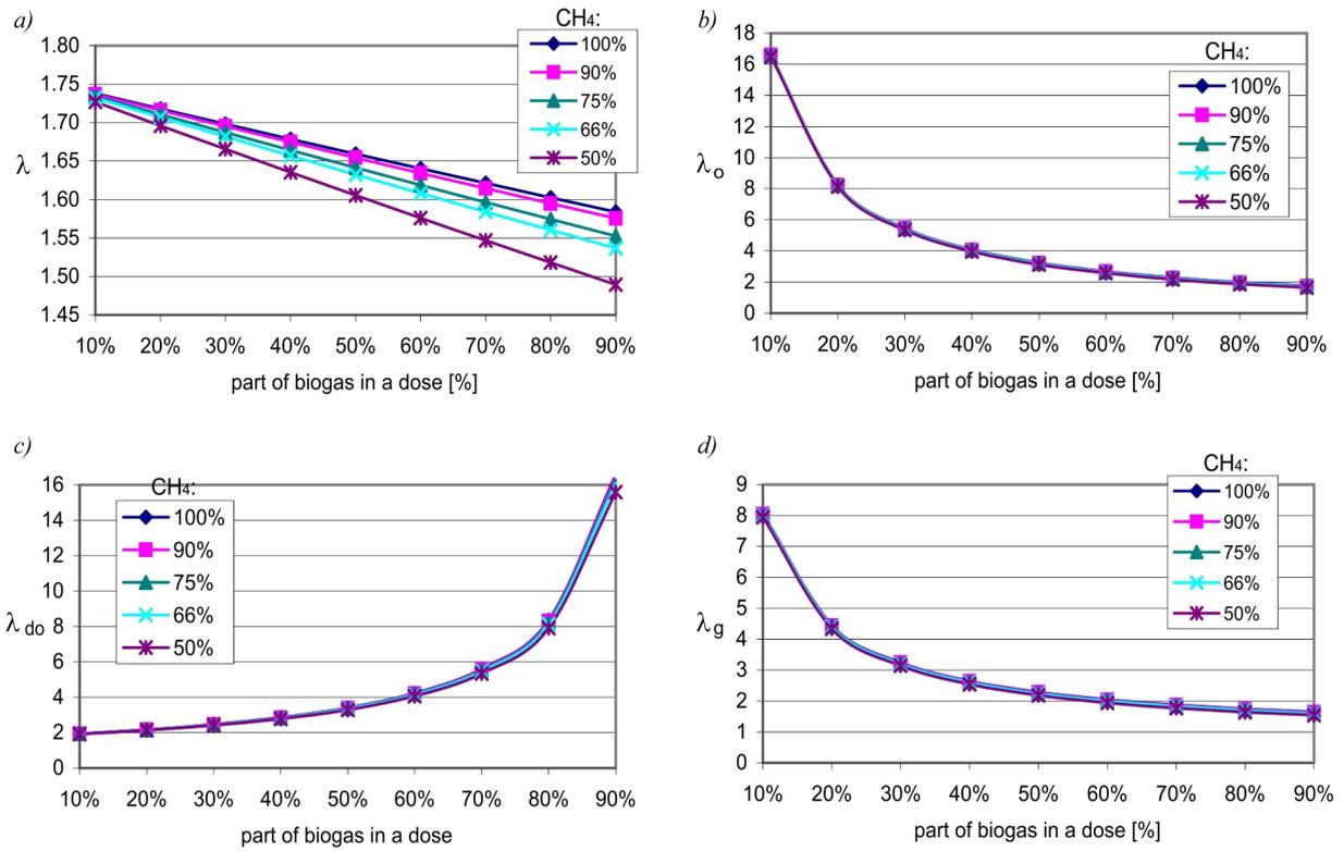
Fig. 2. The impact of the share of biogas in the dose powering the engine for fuels of varying methane content at  $n = 1500 \text{ rpm}$  and  $T = 100 \text{ Nm}$  on the ratios: a)  $\lambda$ , b)  $\lambda_o$  b)  $\lambda_{do}$  b)  $\lambda_g$
