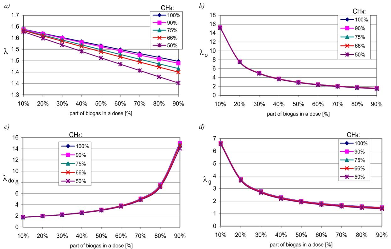
Fig. 3. The impact of the share of biogas in the dose powering the engine for fuels of varying methane content at  $n = 1500 \text{ rpm}$  and  $T = 200 \text{ Nm}$  on the ratios: a)  $\lambda$ , b)  $\lambda_o$  b)  $\lambda_{do}$  b)  $\lambda_g$
