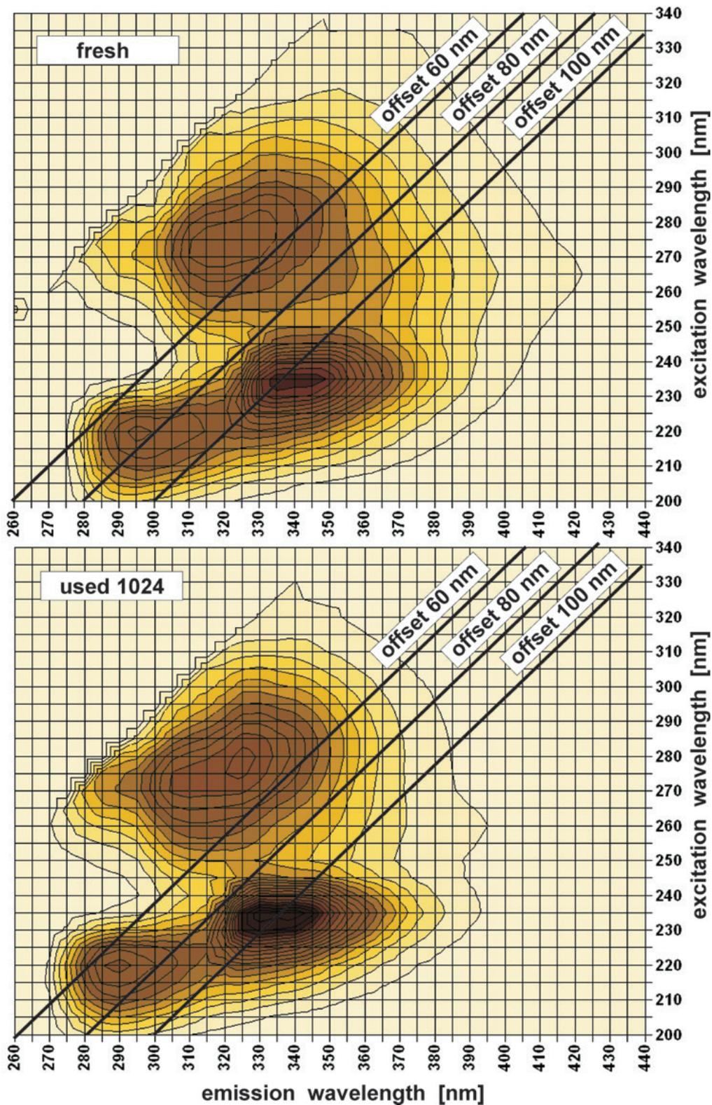
Fig. 2. Excitation-Emission Fluorescence spectra of two used oils: fresh and used one (1224 hours in the engine circuit). Straight diagonal lines show cross-sections resulting in the creation of synchronous fluorescence spectra plotted in Fig. 3
