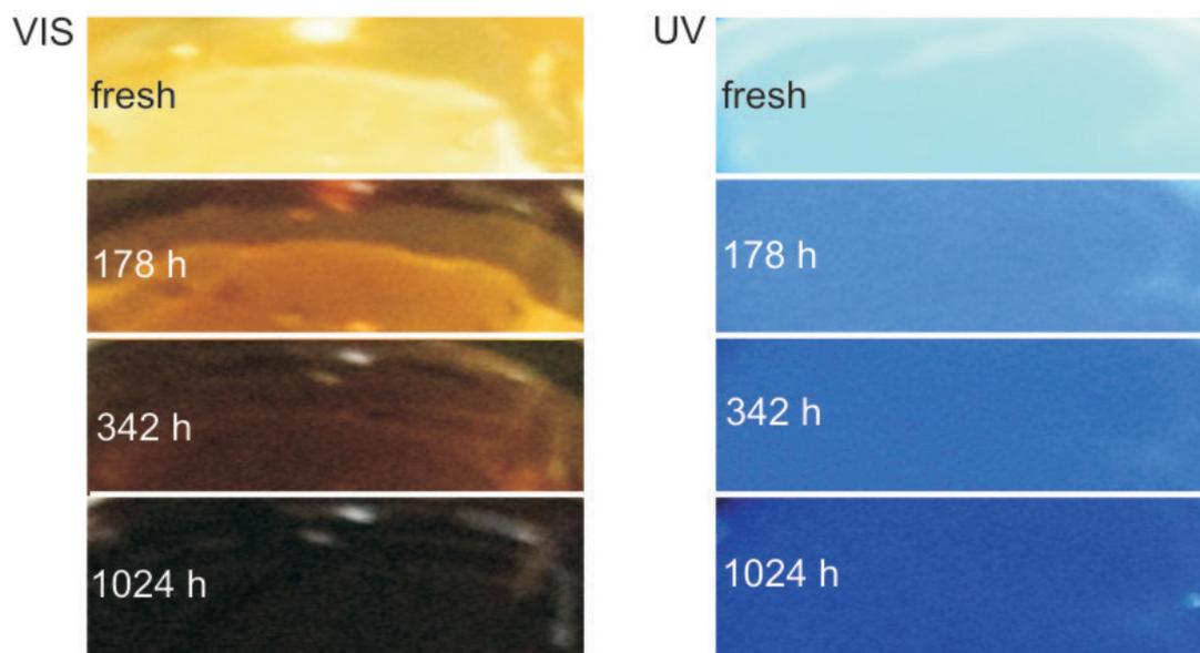
Fig. 1. View of oil samples in visual light (left) and in ultraviolet (right)
