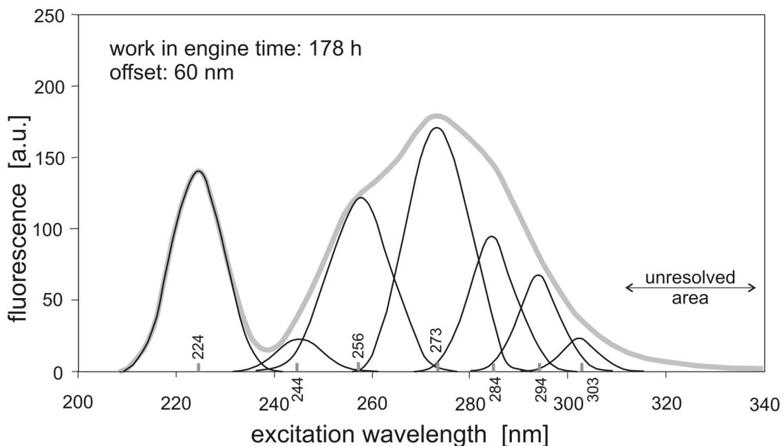
Fig. 4. Exemplary synchronous spectrum been divided into Gaussian curves
