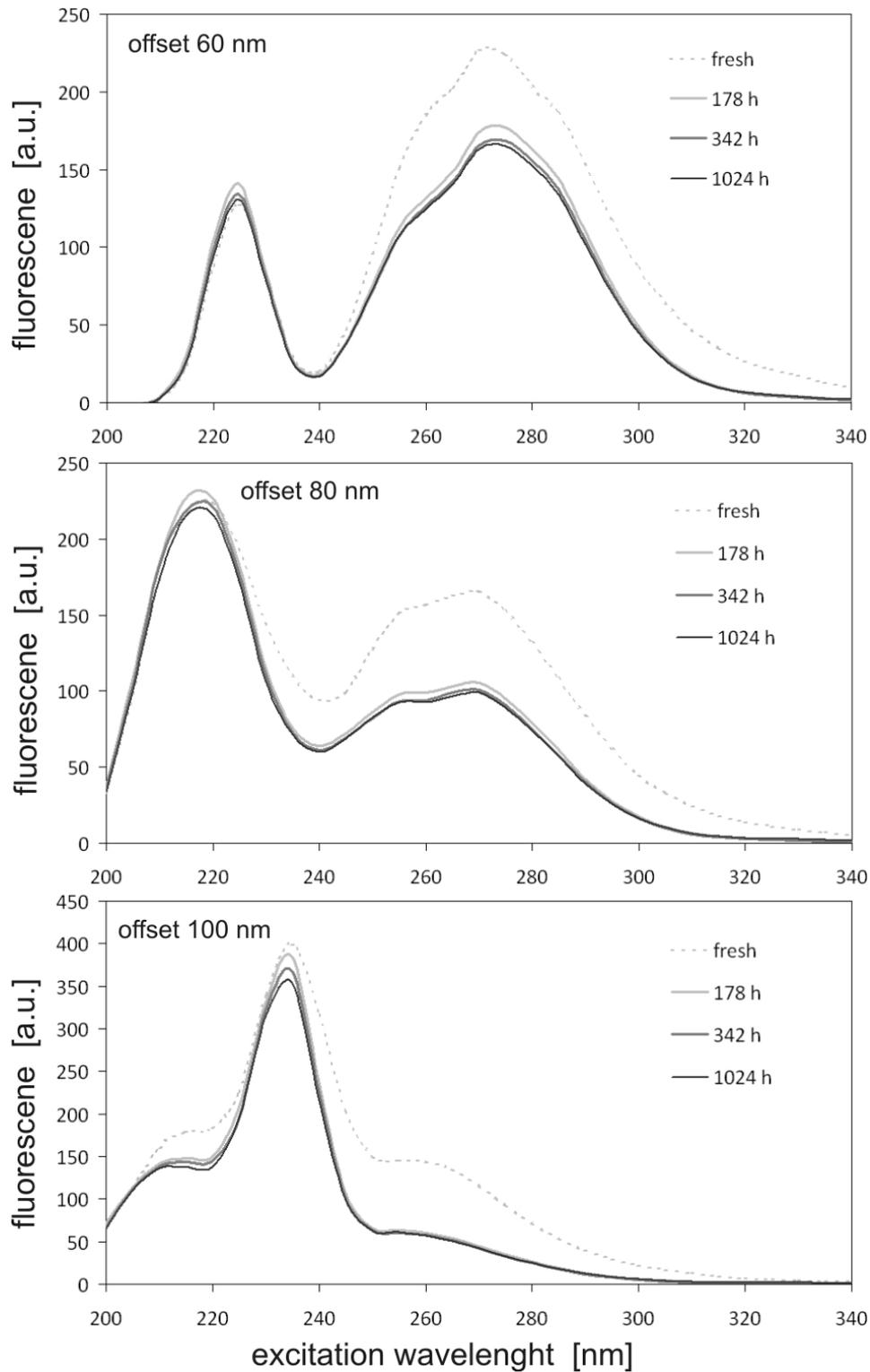
Fig. 3. Fluorescence spectra of oils for constant wavelength internal 60 nm, 80 nm and 100 nm (distance between excitation and emission wavelengths)
