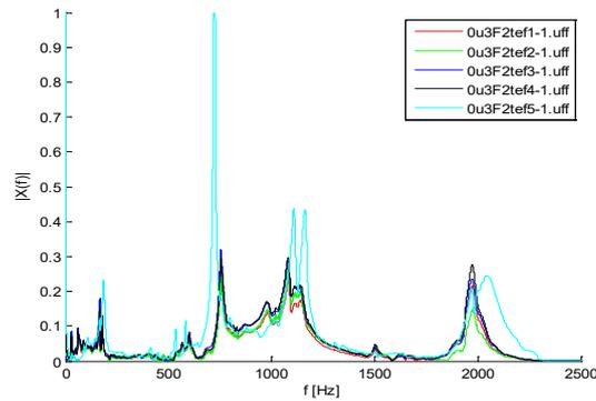
Fig. 4. FFT (ACCI) for five strokes made with Teflon head of impact hammer in impact place F2 for the plate made of homogenous material
