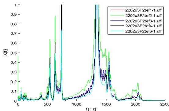
Fig. 6. FFT (ACCI) for five strokes made with Teflon head of impact hammer in impact place F2 for the plate without any faults in weld seam
