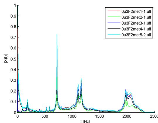
Fig. 3. FFT (ACCI) for five strokes made with metal head in impact place F2 for the homogenous material plate
