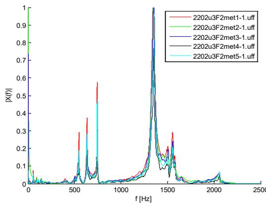
Fig. 5. FFT (ACCI) for five strokes made with metal head of impact hammer in impact place F2 for the plate without any faults in weld seam
