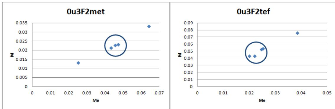
Fig. 7. Dispersion of impact hammer stroke for a homogenous plate
