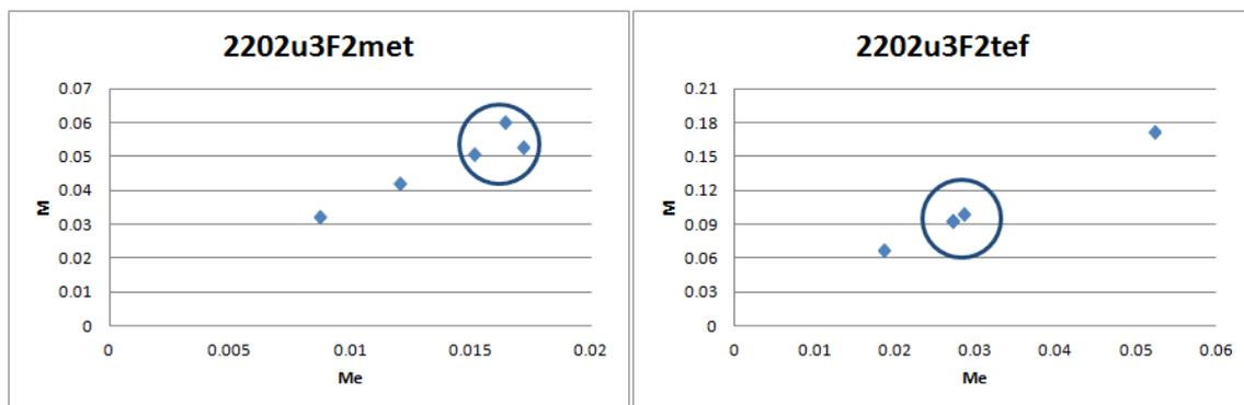
Fig. 8. Dispersion of impact hammer stroke for a welded plate without faults in a seam
