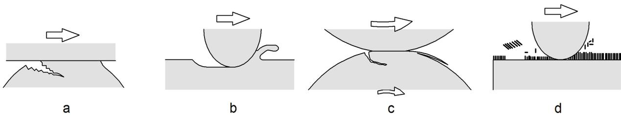
Fig. 1. Selected wear mechanisms (a – adhesive wear, b – abrasive wear, c – fatigue wear, d – corrosion wear) [5]
