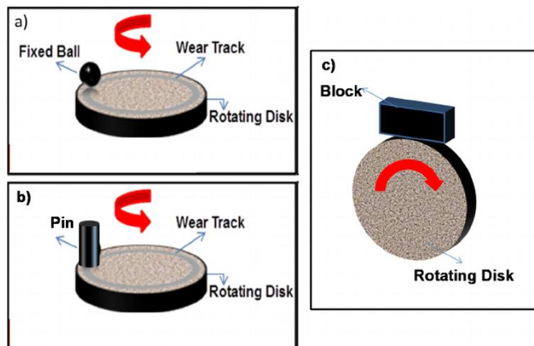
Fig. 2. Most common tribometer configurations [4]
