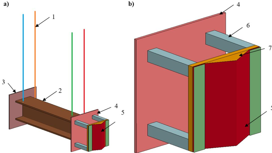
Fig. 2. Ballistic pendulum (a), front part of the pendulum (b), 1 – steel ropes, 2 – double-T beam, 3 – counterweight, 4 – front plate, 5 – deflector; 6 – spacers; 7 – mounting plate
