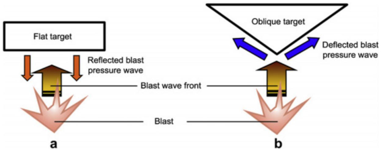
Fig. 1. Schematic of blast wave deflection by flat and V-shaped deflector [2]
