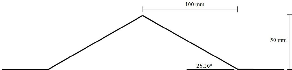
Fig. 3. Geometric shape of tested deflector
