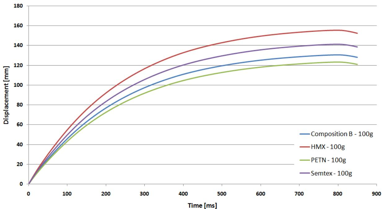
Fig. 5. Time-displacement graph for 100 g explosive materials
