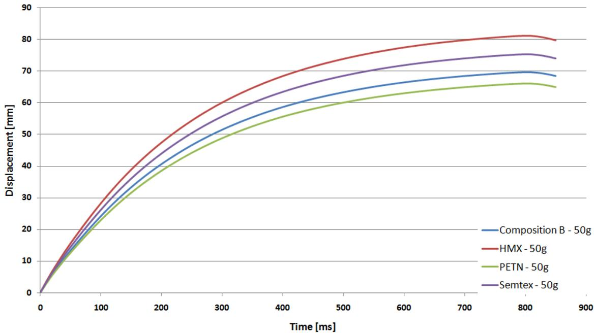
Fig. 4. Time-displacement graph for 50 g explosive materials
