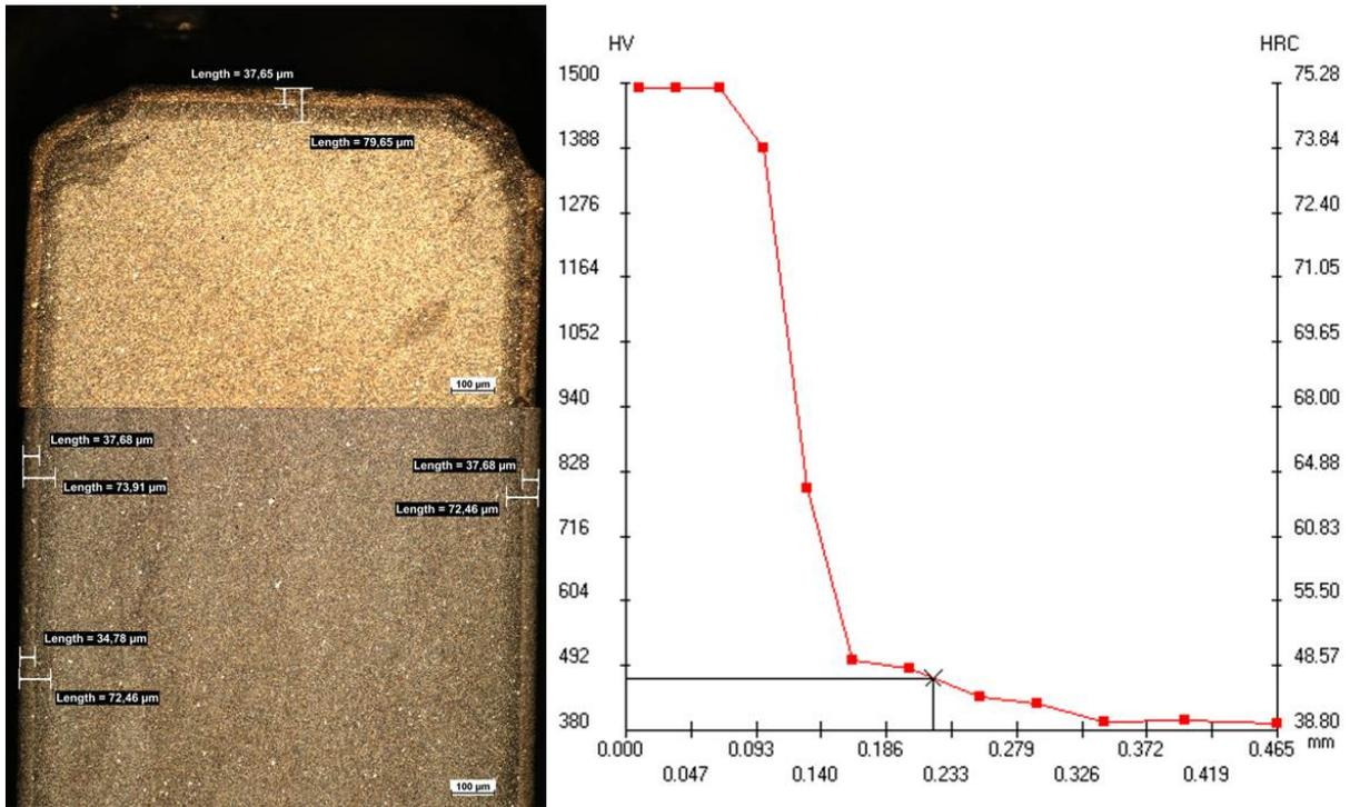
Fig. 2. Microstructure of nitrided piston ring 1-8, x100 (on the left side) and hardness distribution HV0.1 from surface to core (on the right side)
