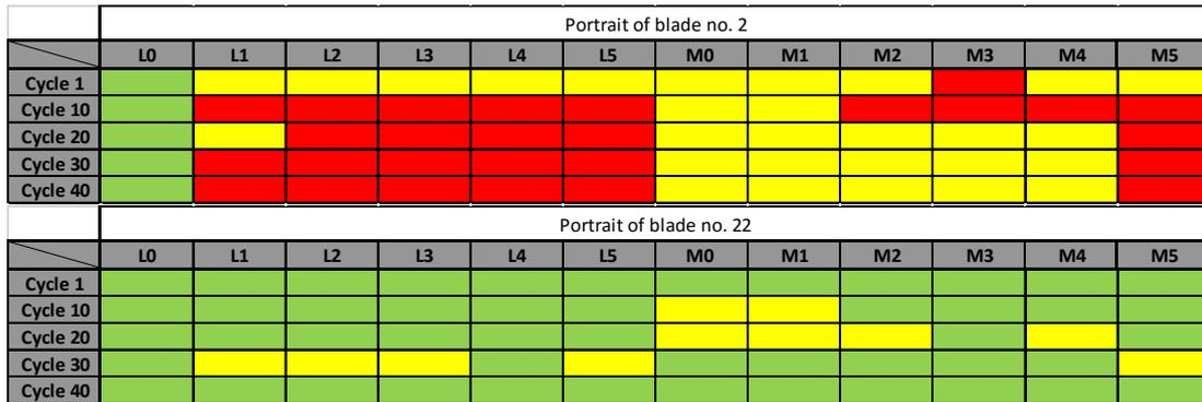
Fig. 2. Portrait of the blades using a model based on auto power spectral densities a) blade no. 2 with increased wear; b) blade no. 22 with normal wear
