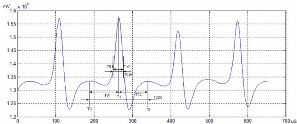
Fig. 1. Inductive sensor signal:  $T_{02d}$ ,  $T_{02k}$  – respectively long and short observation period of blade being in sensor area;  $T_0$ ,  $T_1$ ,  $T_2$  – characteristic observation moments of blade tip below the sensor;  $T_{01}$ ,  $T_{12}$  – observation sub periods of blade tip for  $T_d$  and  $T_k$  respectively;  $mV$  – blade tip translocation signal,  $\mu S$  – blade translocation time [12]
