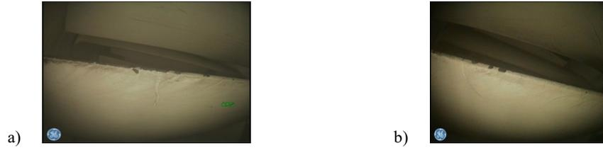
Fig. 4. Selected view of the leading edge of the lock to the top a) blade no. 2; b) blade no. 22 [12]
