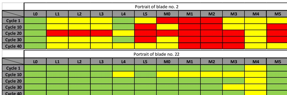
Fig. 3. Portrait of the blades using a model based on cross power spectral densities a) blade no. 2 with increased wear; b) blade no. 22 with normal wear
