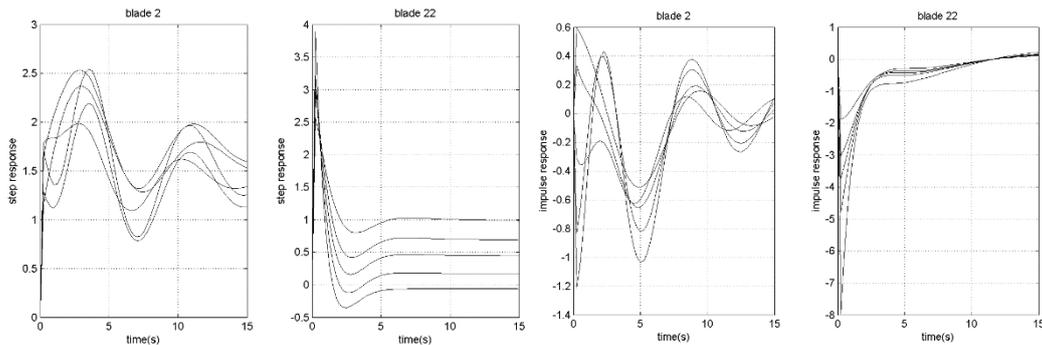
Fig. 7. Impulse and step responses for blades no. 2 and no. 22 for five different cycles
