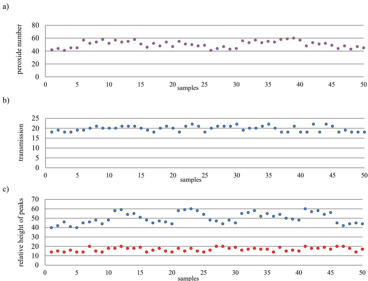
Fig. 4. Distribution of the FAME test results of: a) peroxide number, b) peak height for the wavenumber of  $890\text{ cm}^{-1}$  (infrared spectroscopy method), c) height of the peaks C18:1 and C18:2 (gas chromatography)
