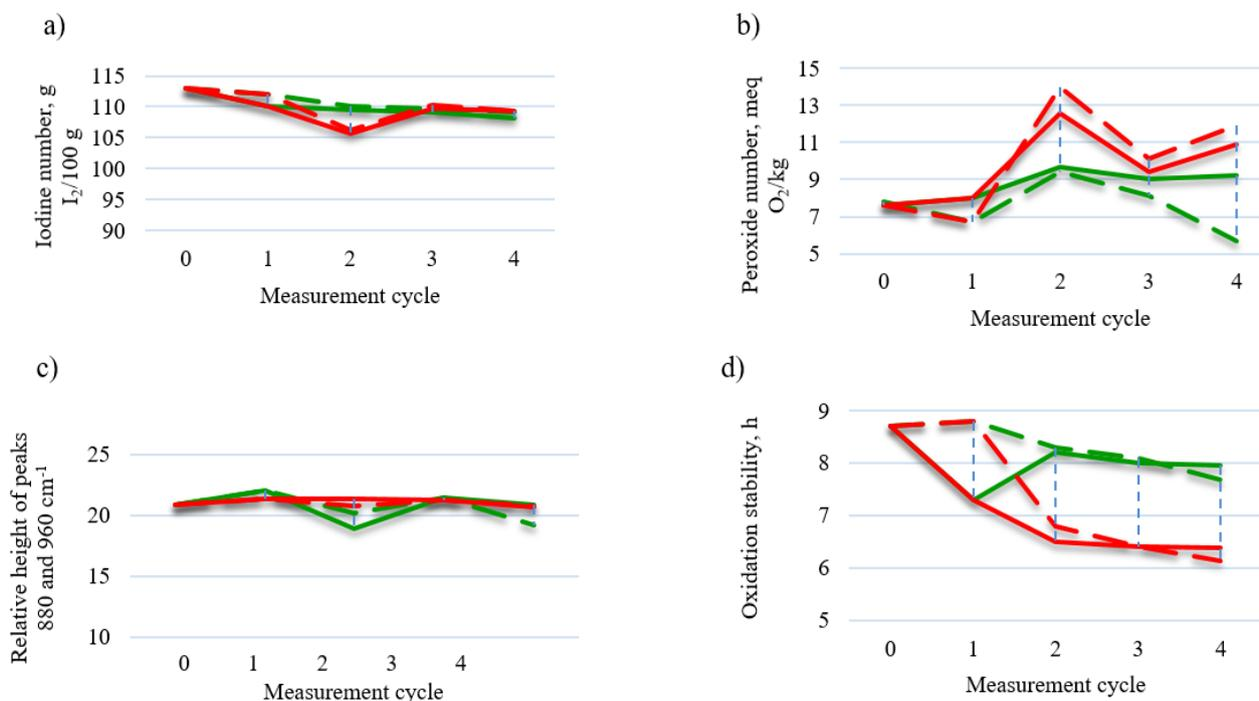
Fig. 6. Course of changes in values of the physical and chemical properties during ageing in simulation tanks: a) iodine number, b) peroxide number, c) relative height of peaks  $880\text{ cm}^{-1}$  and  $960\text{ cm}^{-1}$  in the UV-VIS spectrum, d) oxidation stability (— upper sample without heating, - - lower sample without heating, — heated upper sample, - - heated lower sample)
