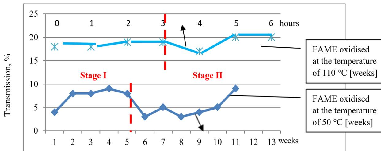
Fig. 5. Comparison of changes in the intensity of the  $890\text{ cm}^{-1}$  band derived from peroxides during the FAME sample storage under different conditions
