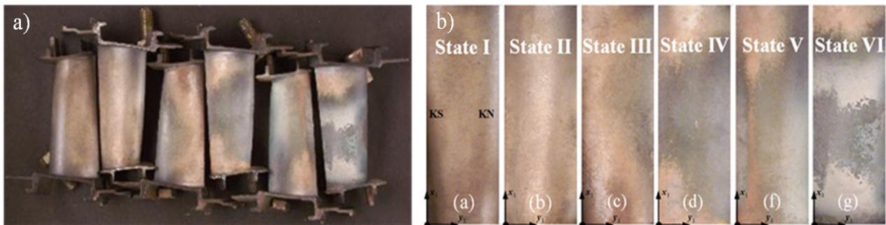
Fig. 2. Nozzle guide vanes of gas turbine: a) image of the surface recorded using a digital camera; b) separate surfaces with the accepted classification according to the state of overheating (a-f)
