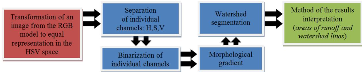
Fig. 4. A block diagram of the procedure used to carry out the image segmentation
