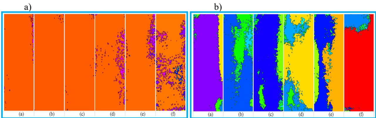
Fig. 5. Exemplary result of the watershed segmentation of the surface images of vanes being in a different technical condition (a-f) – *HSV* model: a) *H* channel; b) *S* channel
