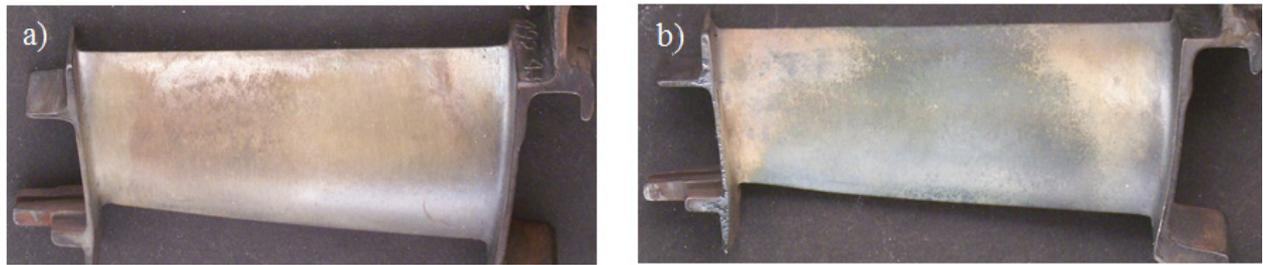
Fig. 1. Stator vanes of the gas turbine (ŻS – 6K alloy) with different degrees of overheating
