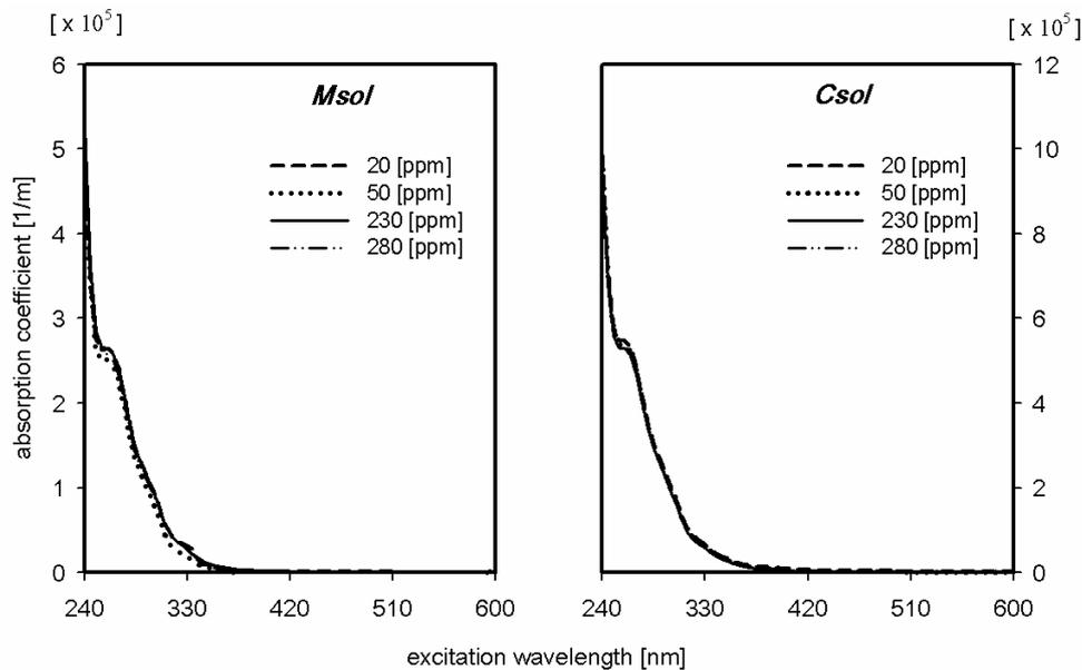
Fig. 2. Absorption coefficient of oil in n-hexane for *Marinol* (*Msol*), *Cyliten* (*Csol*) for various oil concentrations (derived using formula (2) based on the data depicted in Fig. 1)
