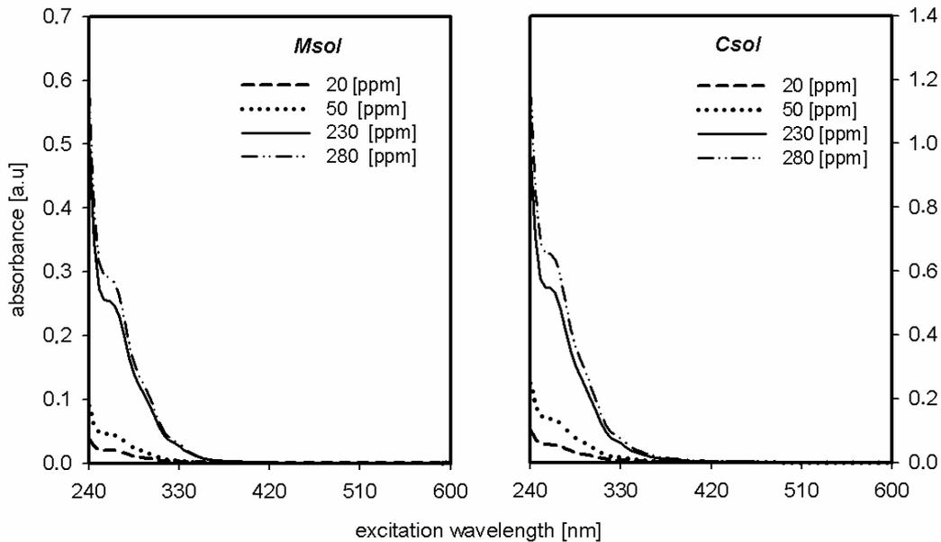
Fig. 1. Absorption spectra of oil in n-hexane for *Marinol* (*Msol*) and *Cyliten* (*Csol*) for various oil concentrations
