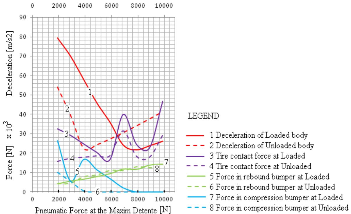
Fig. 5. Evolution of the vehicle body deceleration and of the forces in tire and in rebound and compression suspension stopper bumpers
