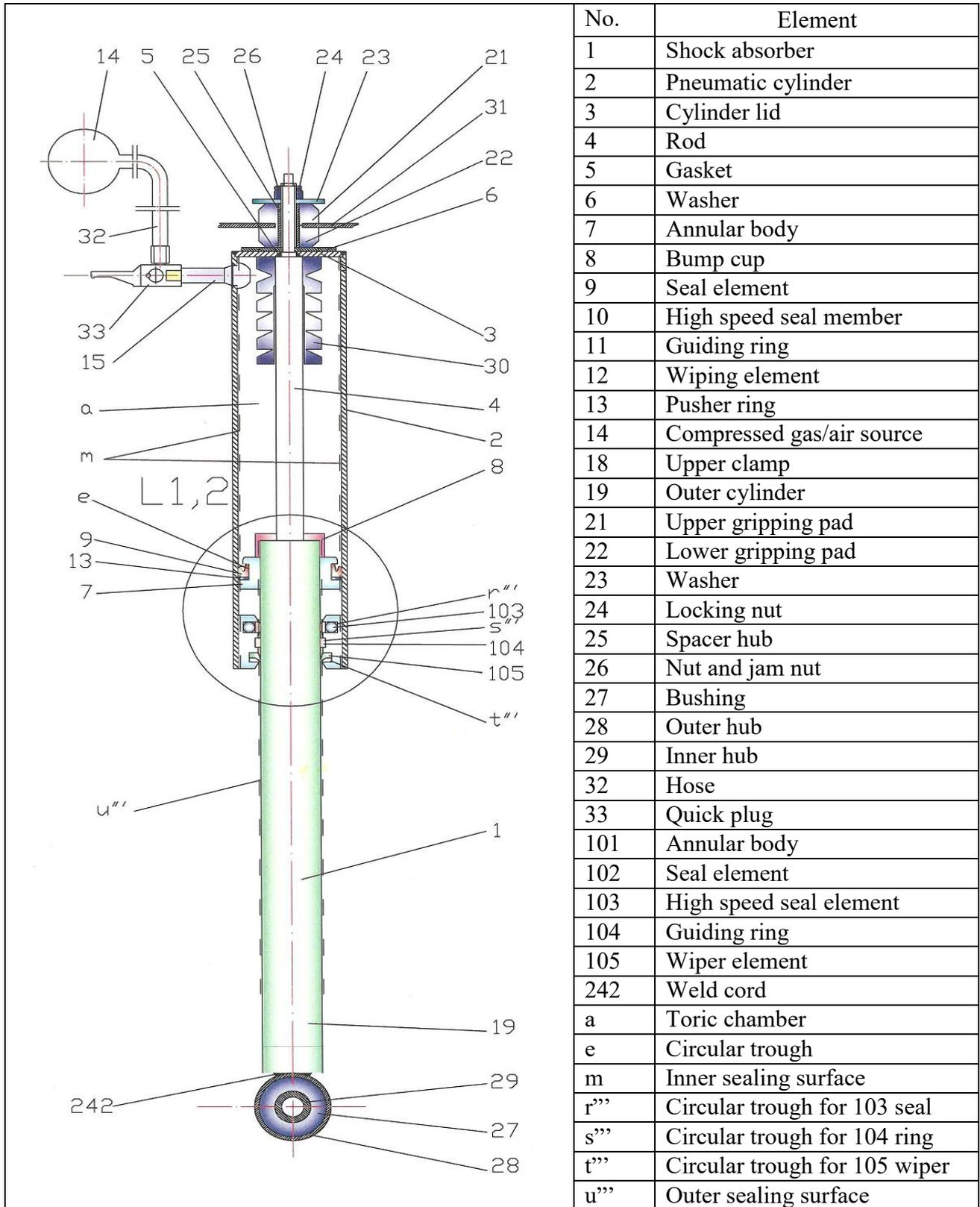
Fig. 1. Shock absorber with cylindrical actuator – version double sliding sealing [1]
