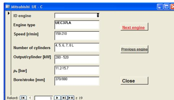
Fig. 7. The form contains data about the parameters of the engine
