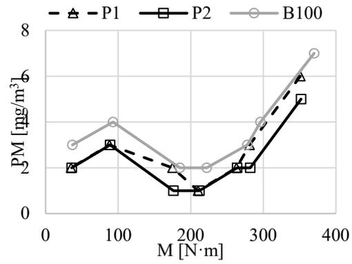
Fig. 10. Dependence of particulate matter concentration on torque change for P1, P2 test fuels and B100 fuel, rotational speed 2,200 rpm
