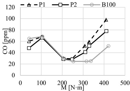
Fig. 3. Dependence of carbon monoxide concentration on torque change for P1, P2 test fuels and B100 fuel, rotational speed 1,400 rpm
