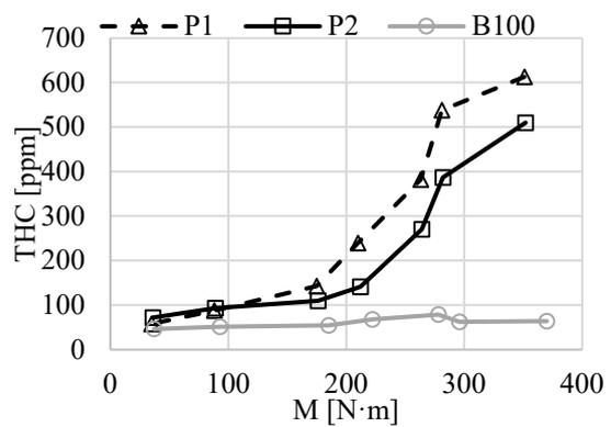
Fig. 8. Dependence of hydrocarbons concentration on torque change for P1, P2 test fuels and B100 fuel, rotational speed 2,200 rpm
