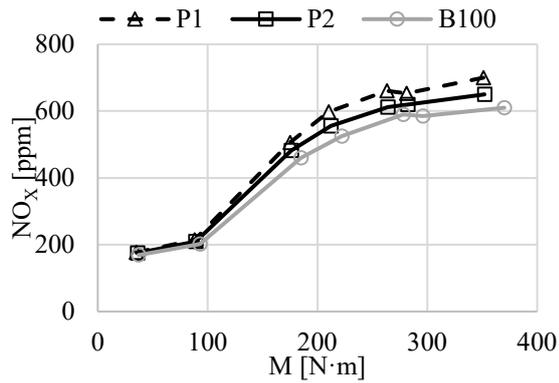
Fig. 9. Dependence of nitric oxides concentration on torque change for P1, P2 test fuels and B100 fuel, rotational speed 2,200 rpm
