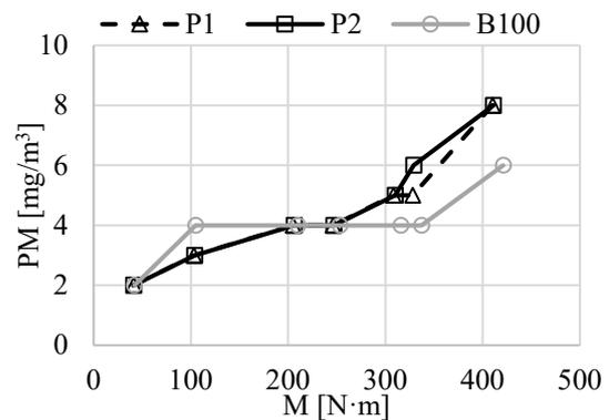
Fig. 6. Dependence of particulate matter concentration on torque change for P1, P2 test fuels and B100 fuel, rotational speed 1,400 rpm
