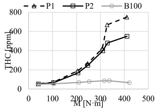
Fig. 4. Dependence of hydrocarbons concentration on torque change for P1, P2 test fuels and B100 fuel, rotational speed 1,400 rpm
