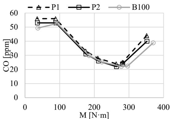
Fig. 7. Dependence of carbon monoxide concentration on torque change for P1, P2 test fuels and B100 fuel, rotational speed 2,200 rpm
