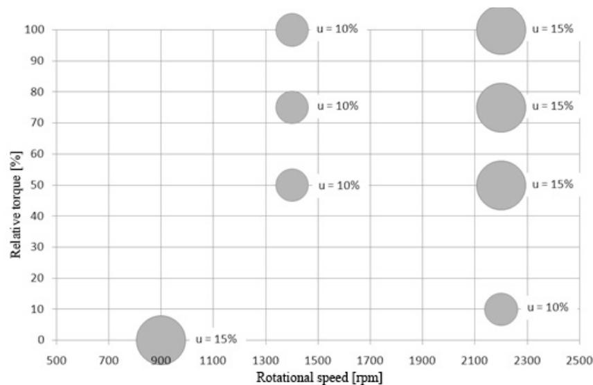
Fig. 2. Weighting factors depending on the rotational speed and load in the C1 test acc. to ISO 8178 standard
