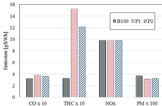
Fig. 11. Examination of toxic substances emission in C1 test as per ISO 8178
