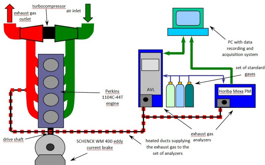
Fig. 1. Block diagram of test station
