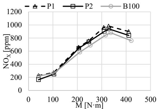
Fig. 5. Dependence of nitric oxides concentration on torque change for P1, P2 test fuels and B100 fuel, rotational speed 1,400 rpm
