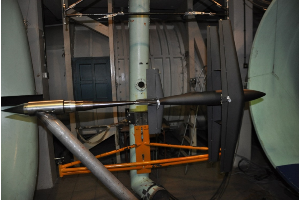
Fig. 4. The model of aircraft „Harnaś 3” in T-1 IoA wind tunnel at rolling angle \varphi = 90^\circ
