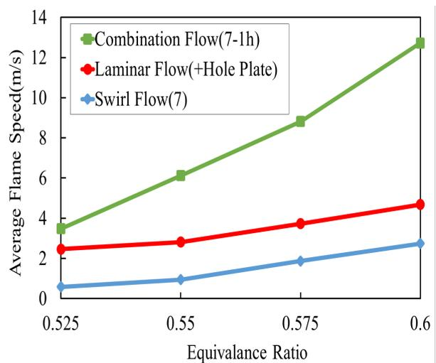
Fig. 5. Average flame speed with combination flow
