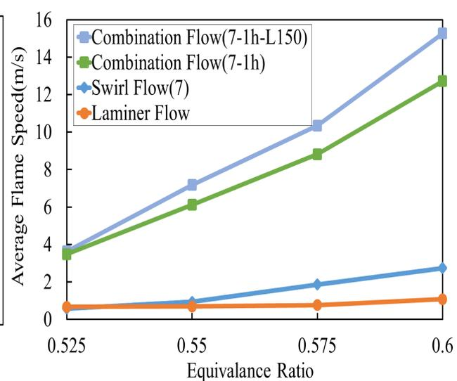
Fig. 9. Average flame speed (Comparison)
