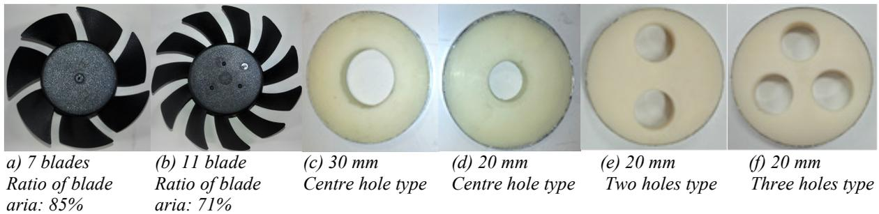
Fig. 2. Experimental blade and plate with hole
