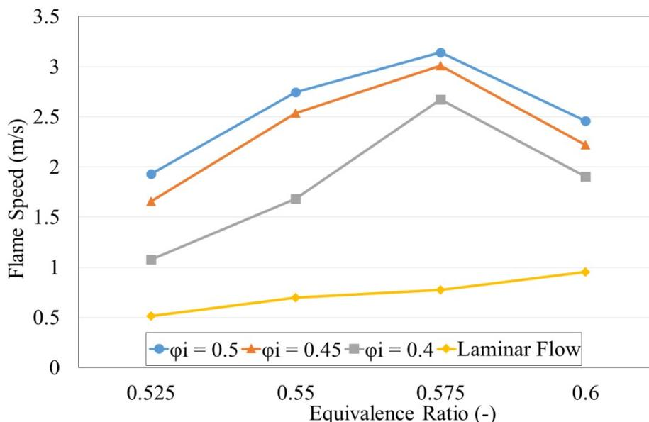
Fig. 11. Flame speed with mixture injection
