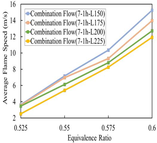
Fig. 7. Average flame speed with combination flow (effects of combination flow intensity)
