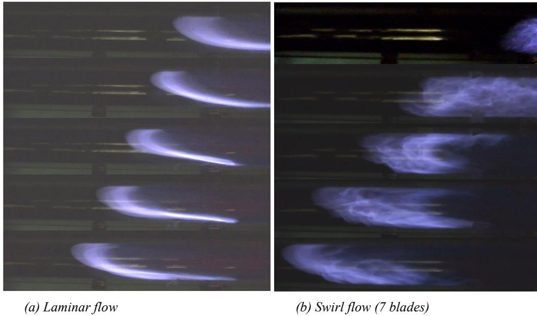
Fig. 3. Flame shape (Propane-air  $\phi = 0.55$ )
