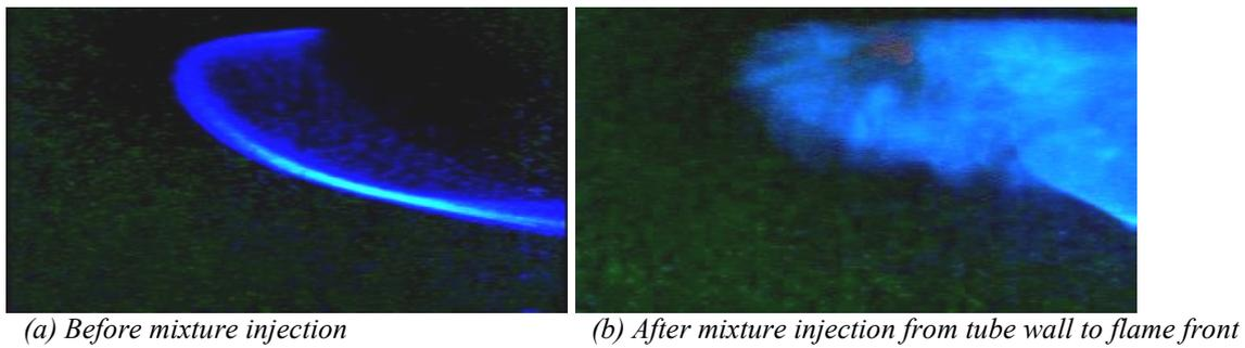
Fig. 10. Flame shape (Propane-air  $\phi = 0.60$ )
