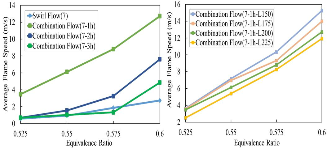
Fig. 6. Average flame speed with combination flow (effects of hole number)      Fig. 7. Average flame speed with combination flow (effects of combination flow intensity)
