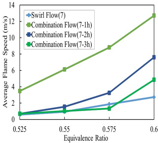
Fig. 6. Average flame speed with combination flow (effects of hole number)
