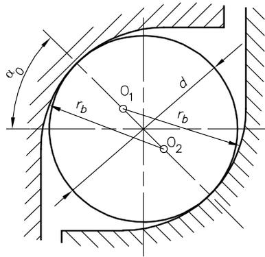
Fig. 1. The race profile of two-row slewing bearing
