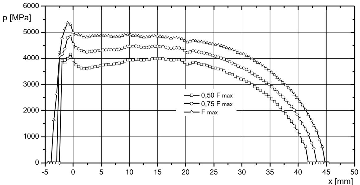
Fig. 3. Distribution of pressure on contact zone of two-row ball slewing bearing for  $k_p = 0.98$ ,  $d = 76.2$  mm,  $F_{max} = 448$  kN, according to [6]
