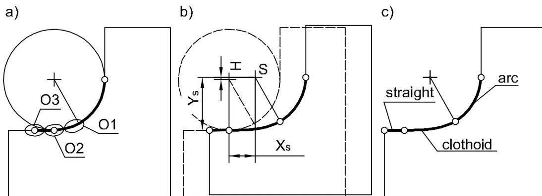
Fig. 4. The designation of the modified profile raceway (a), parameters of the modified profile (b), raceway profile after modification (c)
