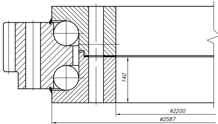
Fig. 5. Two-row ball slewing bearing 2.2P.Z.N.76.2500.0.0.00.C (according to [7])
