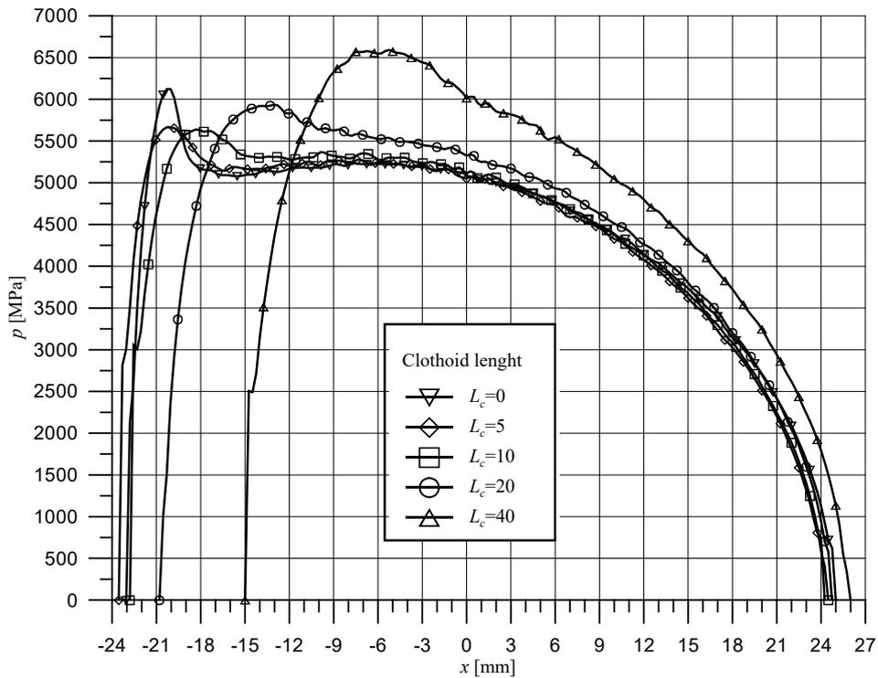
Fig. 8. Pressure distribution on modified profiles for different length of clothoid (for 750 HV)
