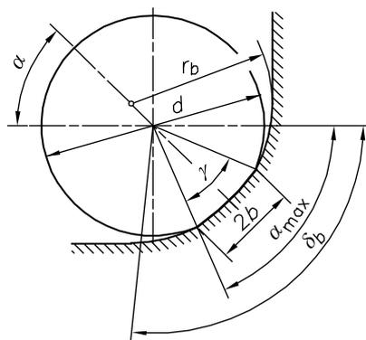
Fig. 2. Schema of contact zone of two-row ball slewing bearing under load:  $\gamma$  – angle of contact area,  $\alpha_{max}$  – angle of scope of contact zone,  $\delta_b$  – angle of race profile
