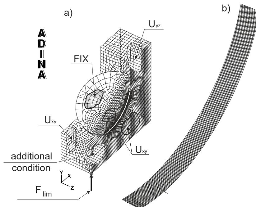
Fig. 6. The mesh of numerical model of contact zone (a) with contact surface (b) – additional condition = identical displacement on Y-axis
