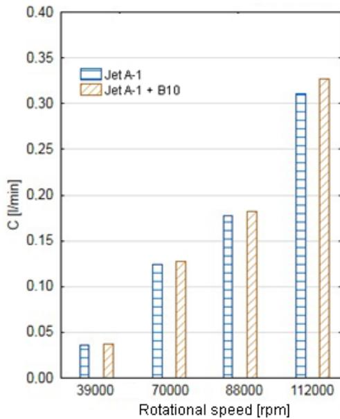
Fig. 4. Fuel consumption as function of rotational speed
