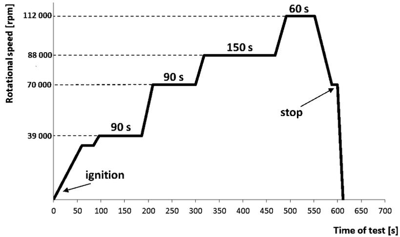
Fig. 1. Operating procedure of engine test
