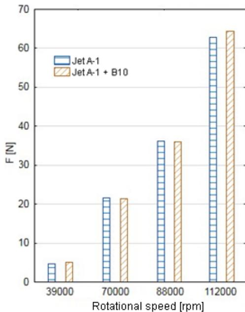
Fig. 2. Thrust as a function of rotational speed
