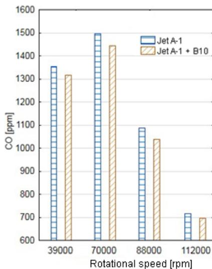
Fig. 6. CO emission as a function of rotational speed
