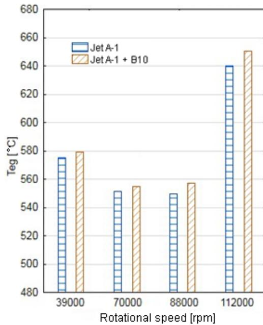
Fig. 3. Exhaust gas temperature as a function of rotational speed
