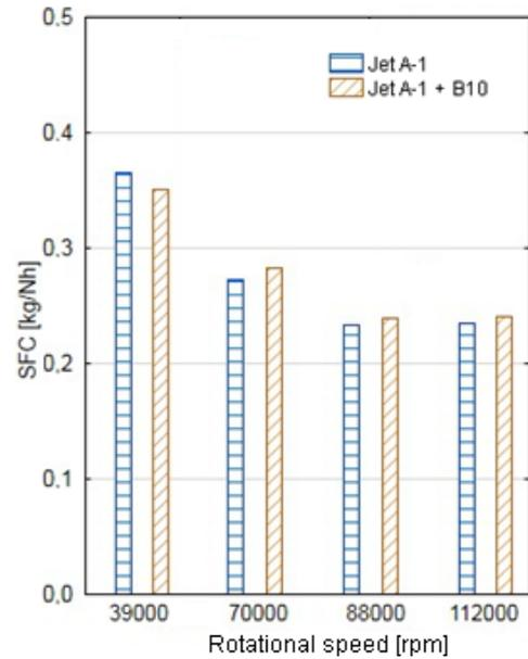
Fig. 5. Specific fuel consumption as a function of rotational speed
