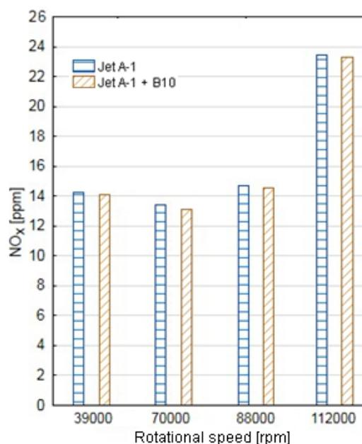
Fig. 8.  $NO_x$  emission as a function of rotational speed
