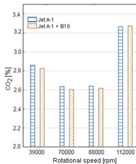
Fig. 7. CO<sub>2</sub> emission as a function of rotational speed
