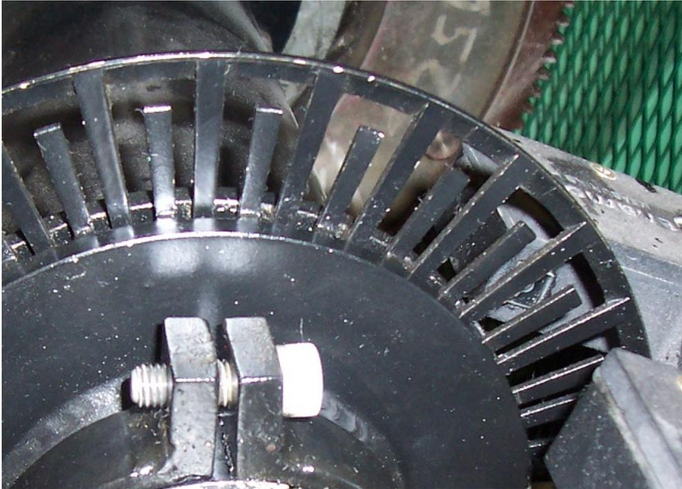
*Fig. 2. Toothed discs for measurement of torque and angular speed*
