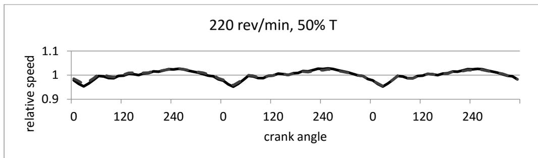
Fig. 5. Fluctuations of relative Instantaneous Angular Speed under 50% of load and 220 rev/min.
