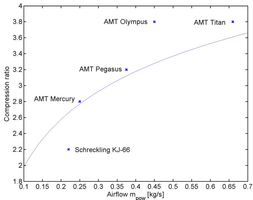
Fig. 4. Single centrifugal stage overall pressure ratio (OPR)
