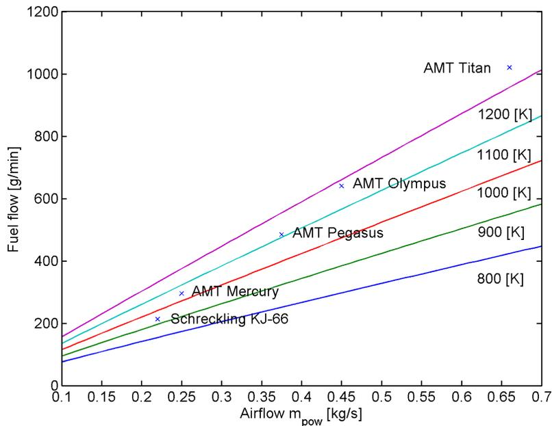
Fig. 10. Identification of microgasturbine fuel consumption
