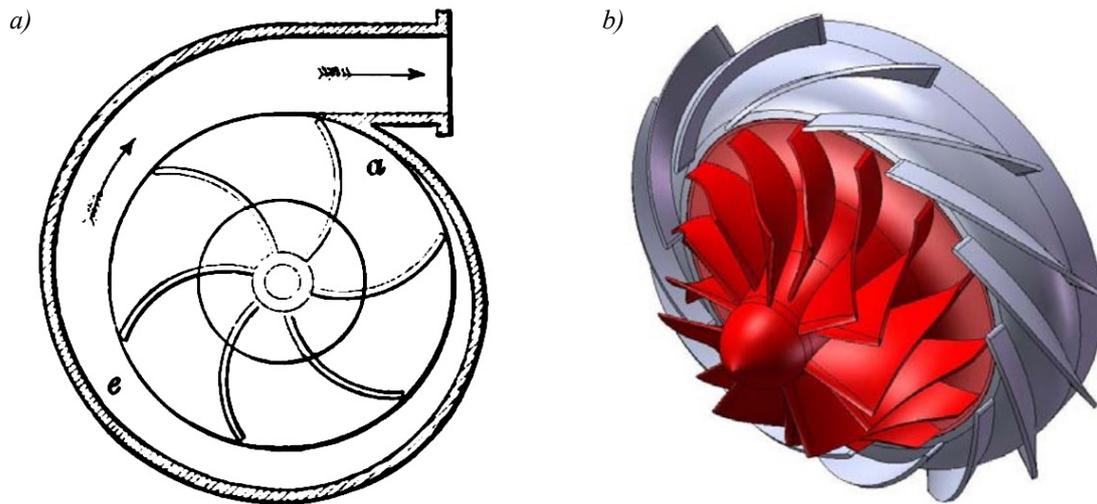
Fig. 5. Centrifugal compressor stage diffuser layout: a) turbocharger, b) turbojet [1]
