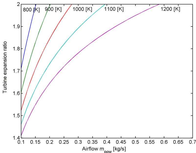
Fig. 8. Identification of microgasturbine turbine expansion ratio  $\Pi_T$
